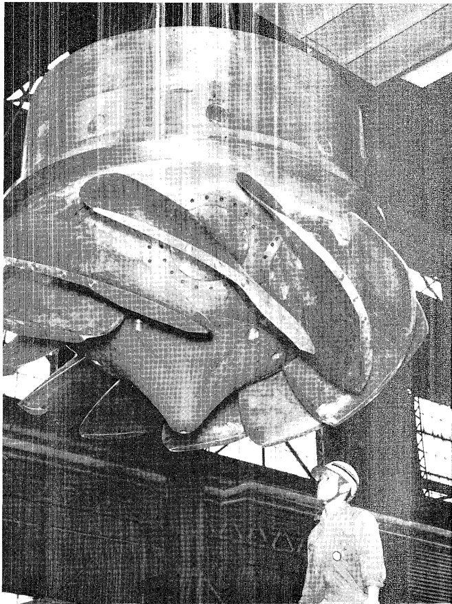
Two-speed Deriaz type pump-turbine for Kuromatagawa No. 2 Power Station
