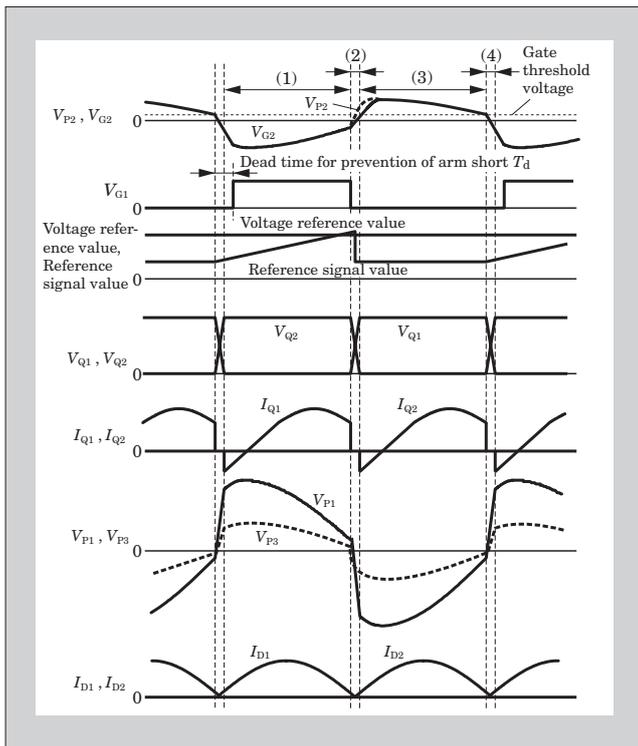
neously and a short-circuit current from flowing. Also, with Q2 in an ON state, a current, inverted from that of period (1), flows to P1 and supplies power to the load.
