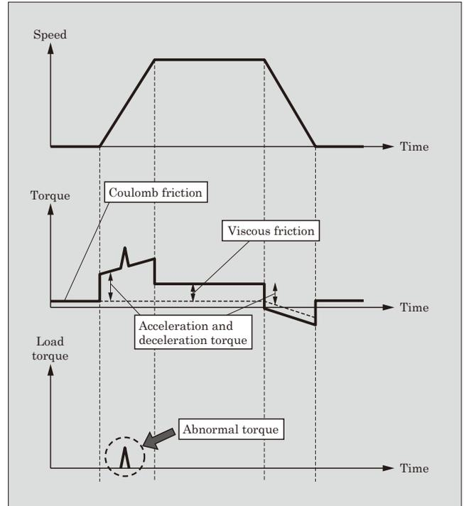
Fig.10 Speed, motor torque and load torque waveforms
