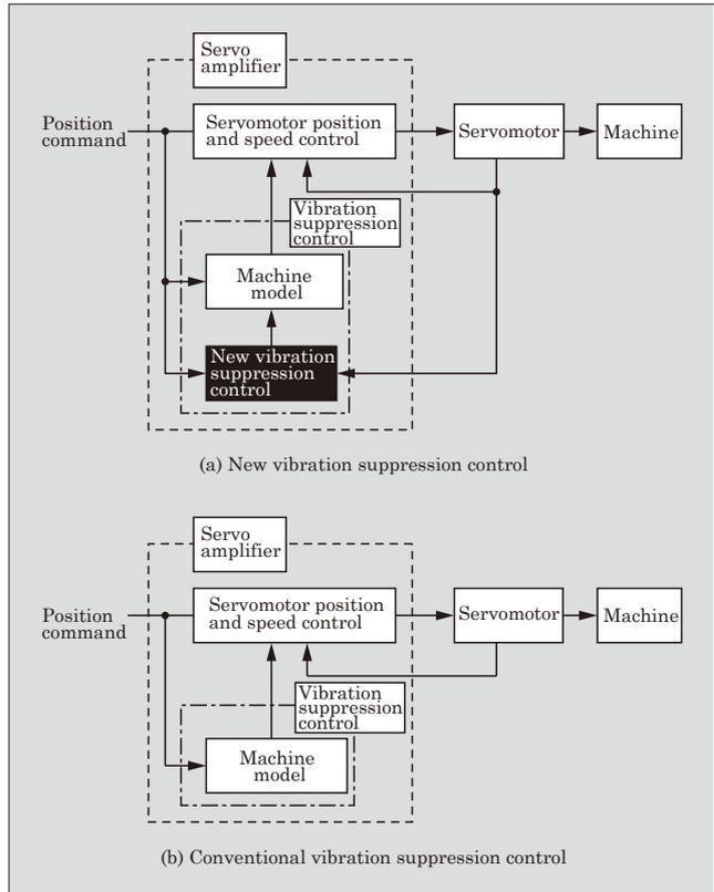
Fig.6 Comparison between block diagrams of new and conventional vibration suppression control
