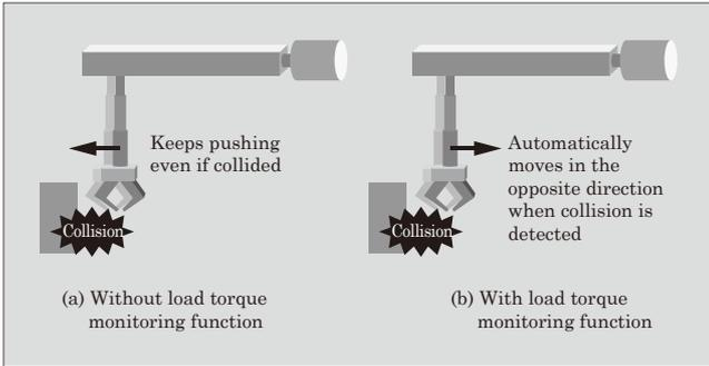
Fig.11 Interference detection by load torque monitoring function
