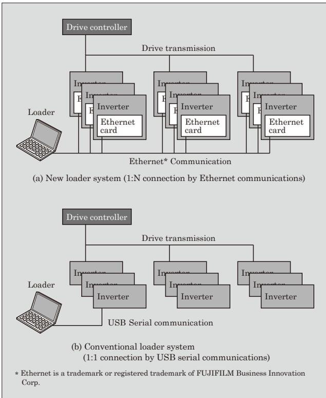
Fig.3 Loader connection
