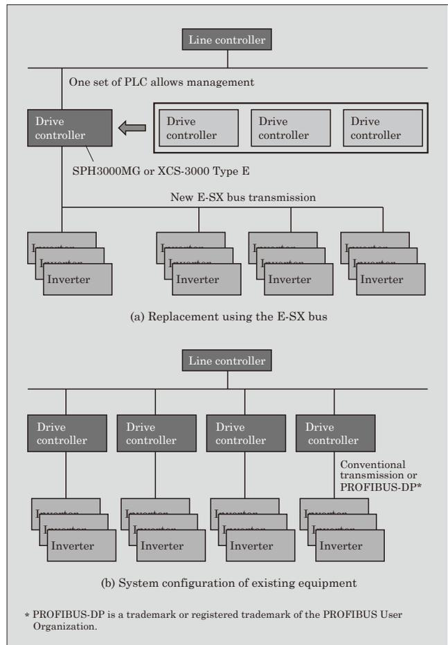
Fig.4 Example of replacement in steel process line
