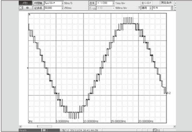
Fig.9 Output voltage waveform during multi-level PWM control (3.3-kV series: between U and V lines)
