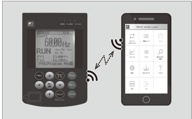
Fig.8 External appearance and Bluetooth connection of the new multi-function keypad
