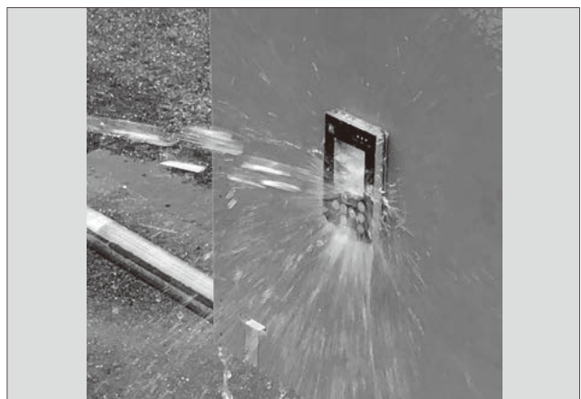
Fig.9 Water resistance test scene of the new multi-function keypad
