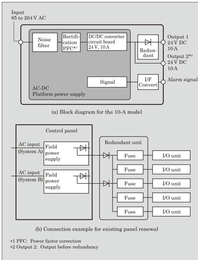
Fig.4 Block diagram and connection example for existing panel renewal
