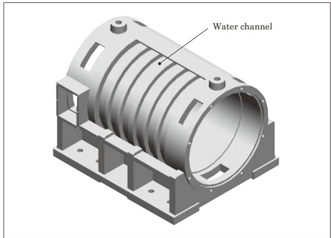
Fig.6 Example of frame in the jacket method
