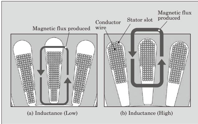
Fig.8 Winding position control
