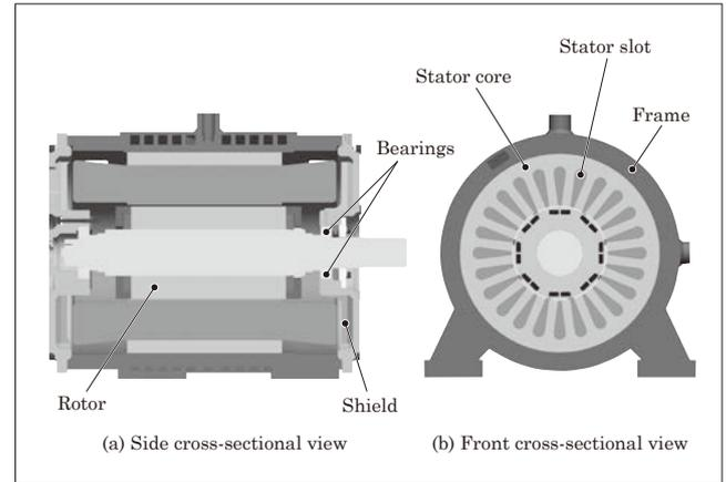
Fig.3 Structural cross-sectional view of PM motor for fluid apparatus
