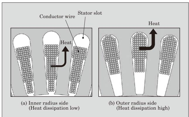
Fig.7 Heat irradiation performance
