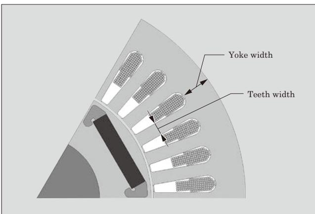
Fig.5 Optimization of teeth and yoke widths
