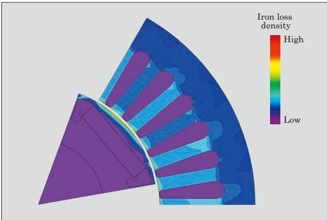
Fig.4 Analysis result of iron loss at the teeth and yoke
