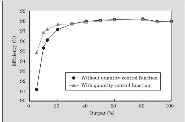
Fig.5 PCS efficiency curve
