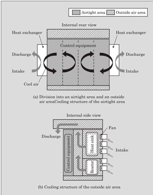
Fig.6 PCS cooling structure
