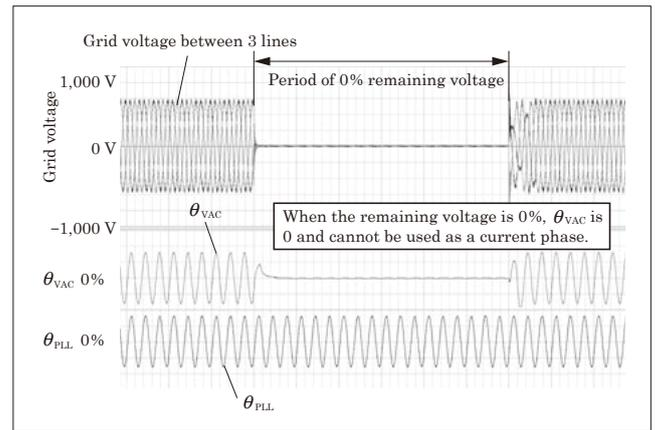
Fig.8 Comparison of current phase  $\theta$  at voltage drop
