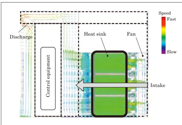
Fig.7 Wind velocity simulation result
