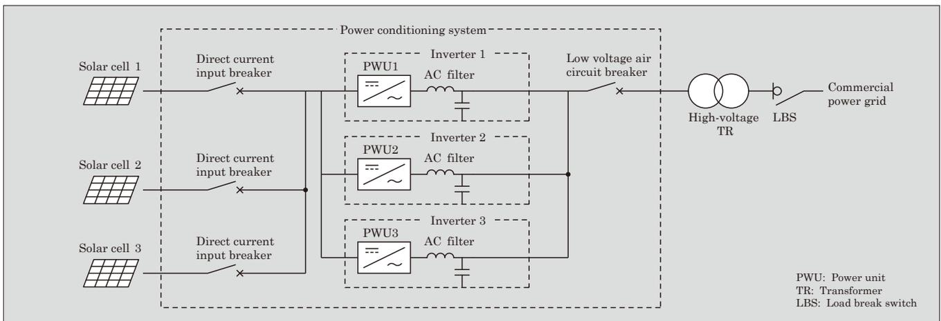
Fig.2 PCS circuit configuration
