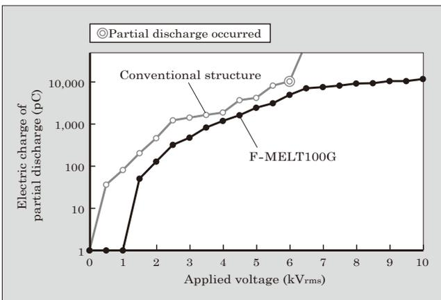
Fig.5 Comparison of occurrence and electric charge of partial discharge depending on the insulation method
