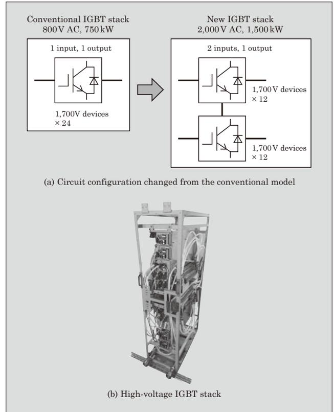
Fig.6 High-voltage IGBT stack and its circuit configuration
