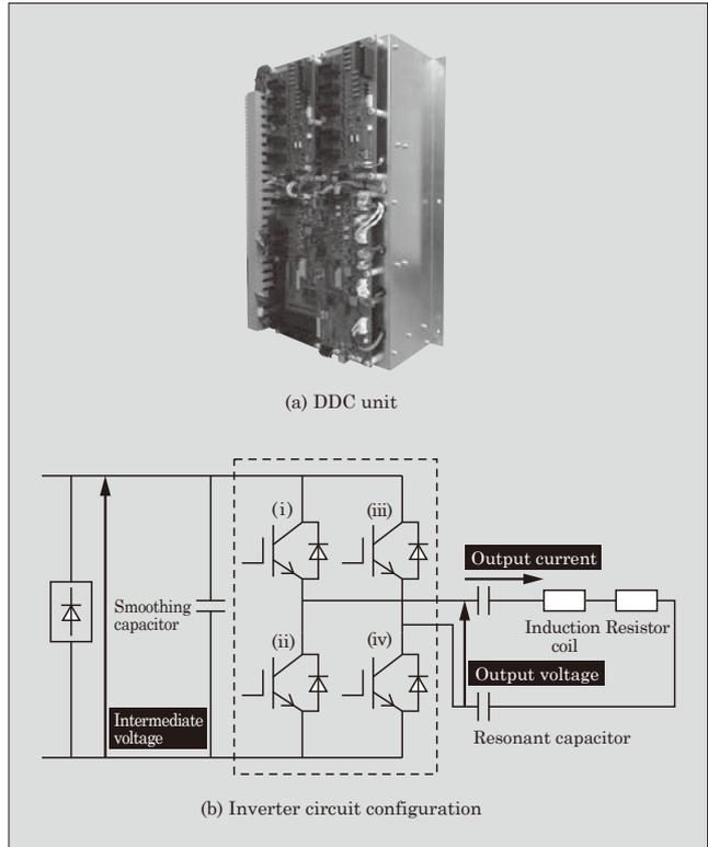
Fig.9 Features of the direct digital control (DDC) unit
