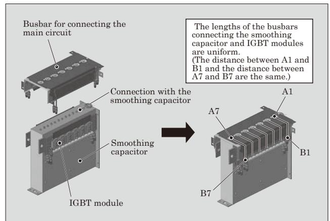
Fig.7 Locations of IGBT modules and smoothing capacitor
