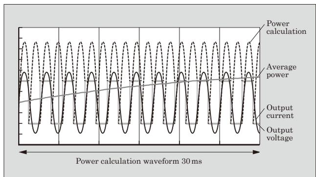
Fig.10 Waveform of high-speed power calculation
