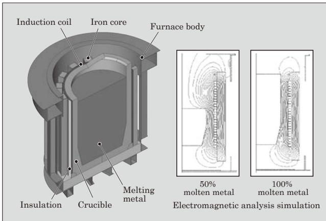
Fig.2 Furnace body structure and electromagnetic analysis simulation example
