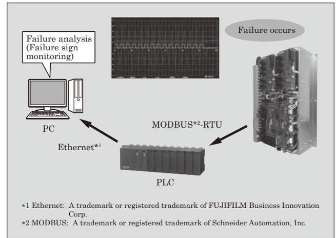
Fig.11 Remote monitoring function (connection of the DDC unit and a PLC)
