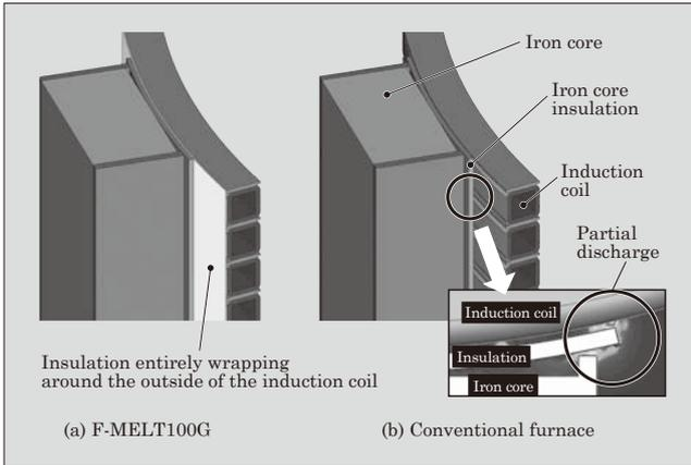
Fig.4 Location of partial discharge
