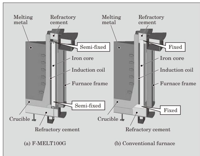
Fig.3 Comparison of iron core fixing structures
