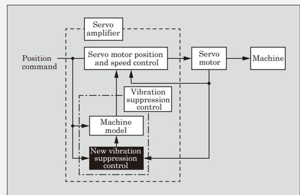
Fig.5 Block diagram of new “ALPHA7 Series” vibration suppression control system
