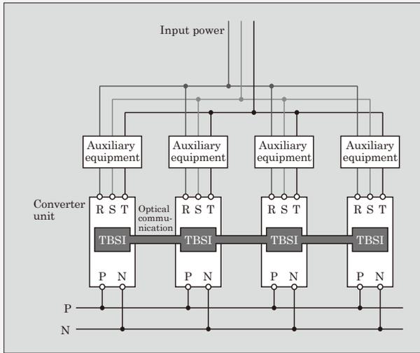
Fig.4 Configuration of the “FRENIC-RHC Series” transformerless parallel system
