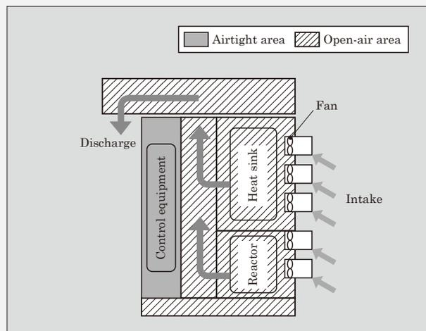
Fig.3 Cooling structure of PCS for mega solar
