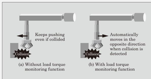
Fig.6 Interference detection using the load torque monitoring function of the "ALPHA7 Series"
