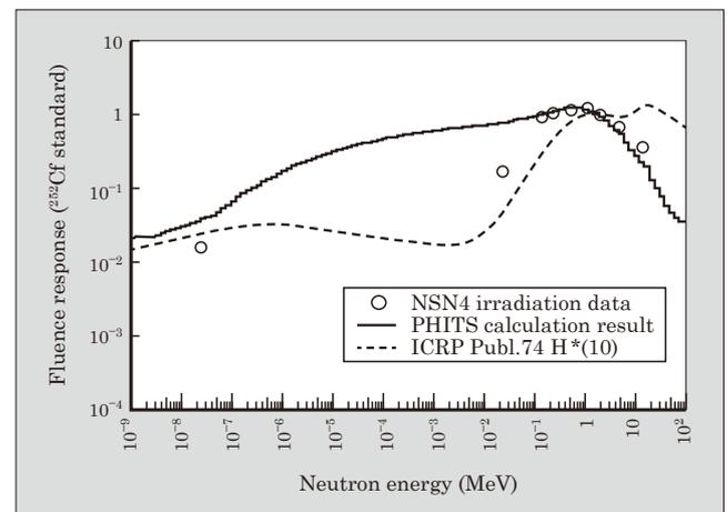
Fig.4 Fluence response to monochromatic energetic neutrons
