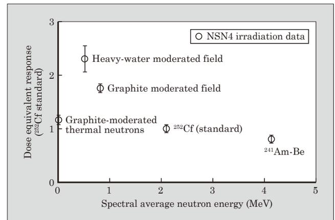
Fig.3 Ambient dose equivalent response to continuous-energy neutrons
