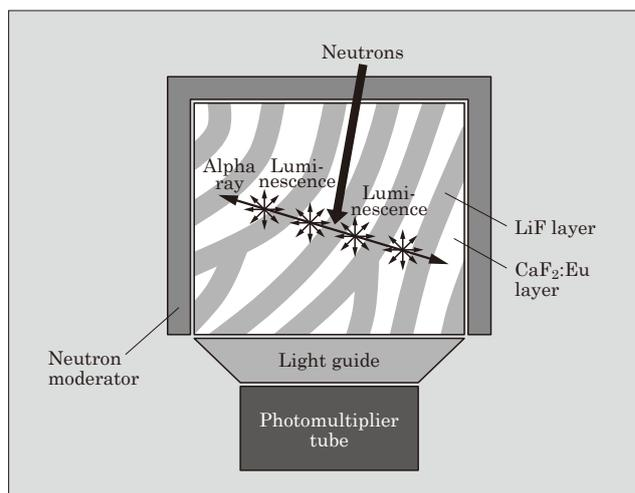
Fig.2 Conceptual diagram of the “NSN4” measurement principle
