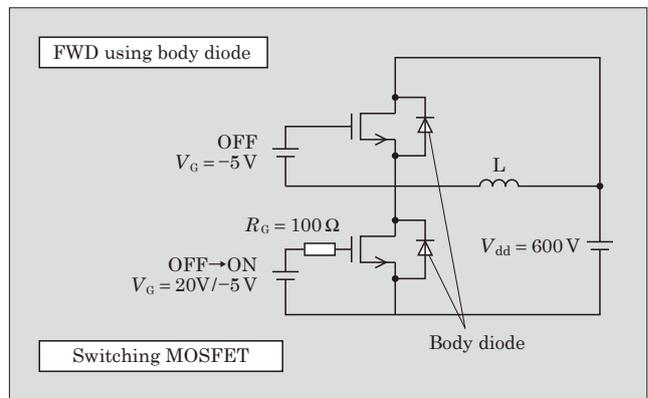
Fig.9 Measurement circuit of reverse recovery
