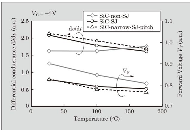
Fig.8 Temperature dependence of  $di/dv$  and  $V_F$  of the body diodes
