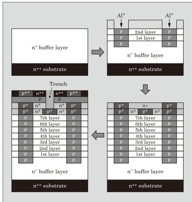
Fig.3 Fabrication flow of SiC-SJ MOSFET
