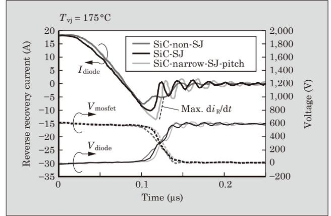
Fig. 12 Comparison of the body diode reverse recovery waveforms
