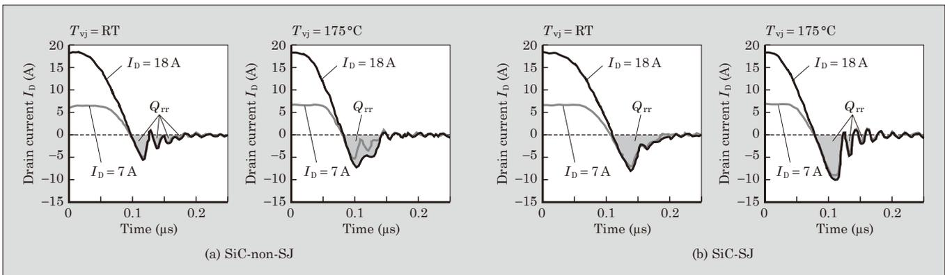
Fig.10 Body diode reverse recovery waveform
