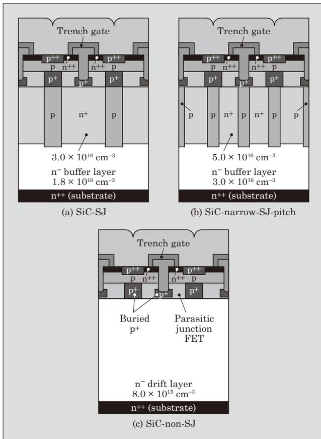
Fig.2 Schematic diagrams of fabricated devices
