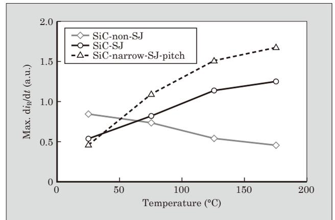
Fig. 13 Temperature dependence of max  $di_R/dt$
