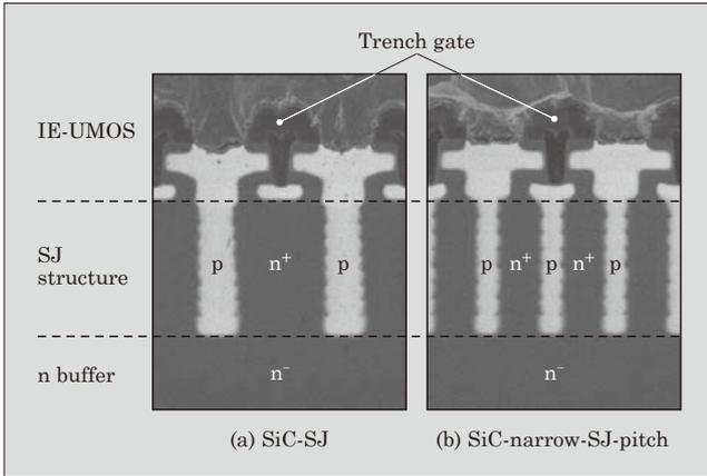
Fig.4 Cross-sectional SEM micrographs of fabricated SJ MOSFETs
