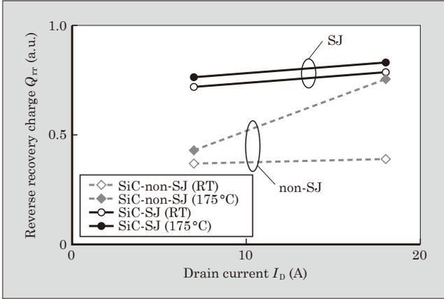
Fig. 11 Current dependence of  $Q_{rr}$  of the body diodes
