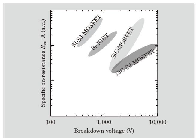
Fig.1 Trade-off relationship between specific on-resistance and blocking voltage
