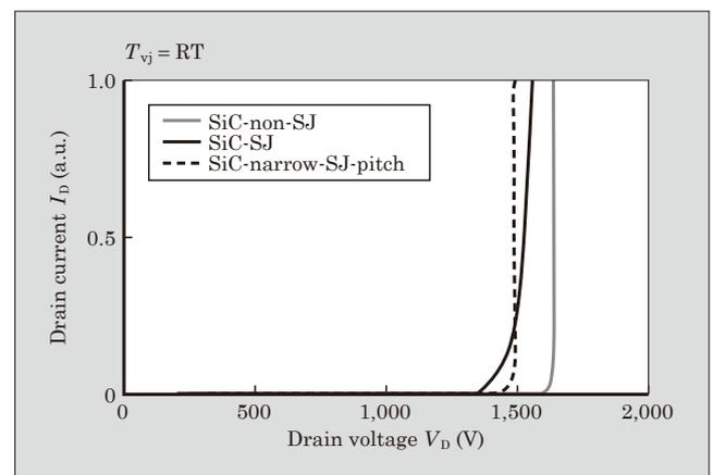
Fig.6 Blocking voltage waveform
