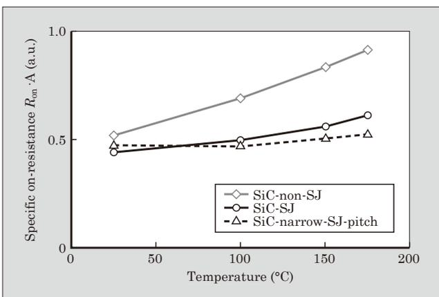
Fig.5 Temperature dependence of specific on-resistance
