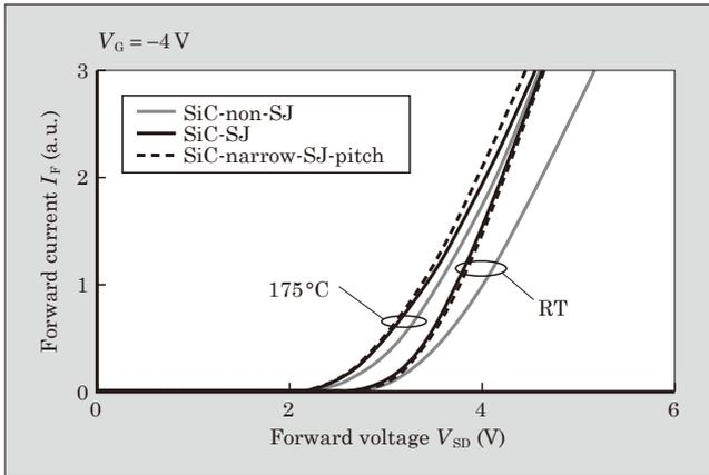
Fig.7 Body diode  $I_F$ - $V_{SD}$  characteristics
