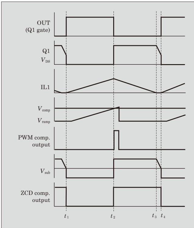
Fig.4 Waveforms of respective parts in switching operation
