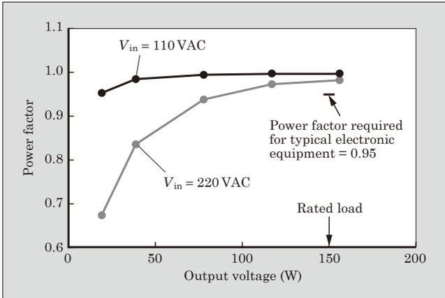
Fig.9 Power factor characteristics
