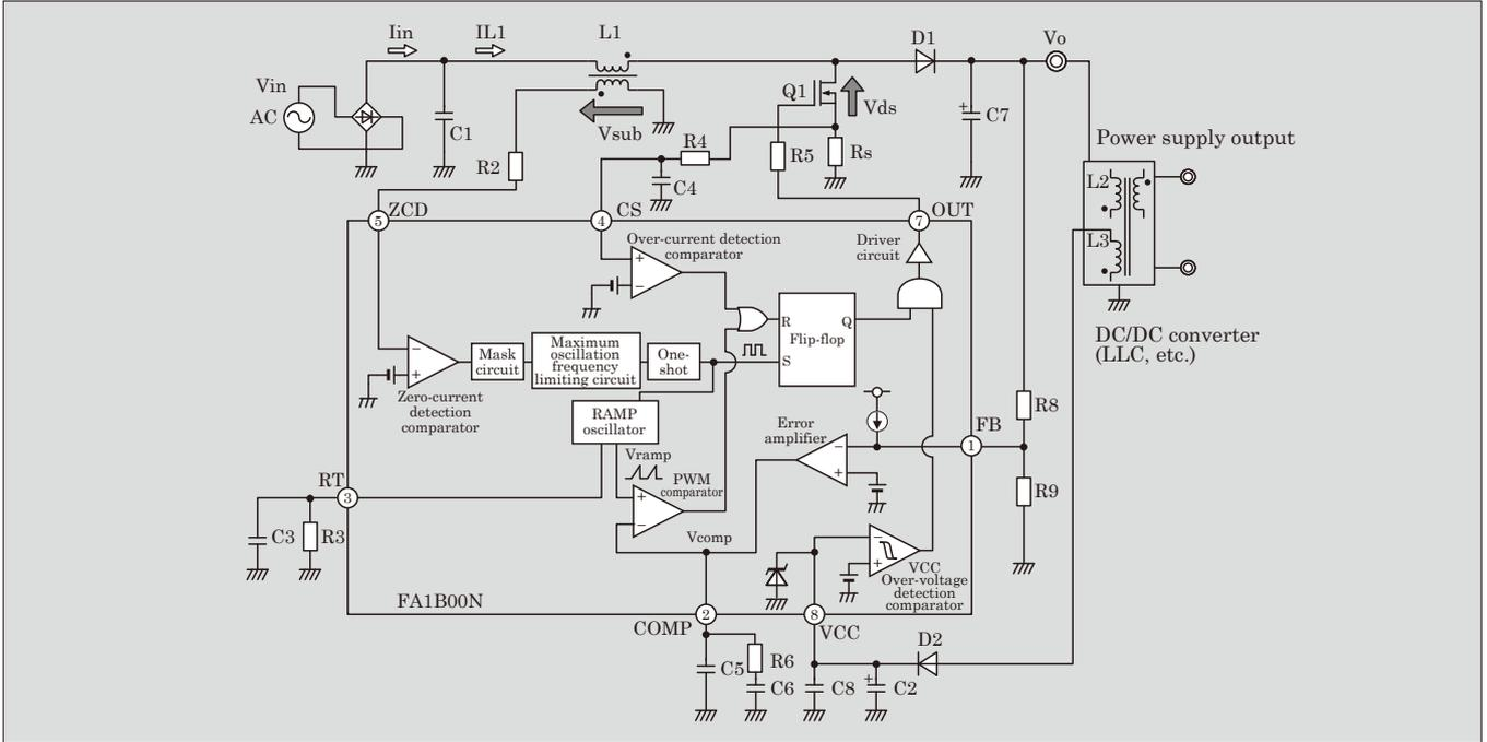
Fig.3 Schematic operation circuit
