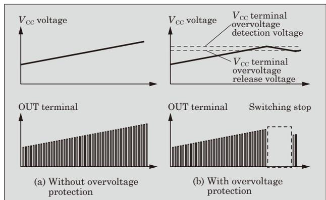
Fig.7 Operation waveform of the overvoltage protective function for  $V_{CC}$  voltage
