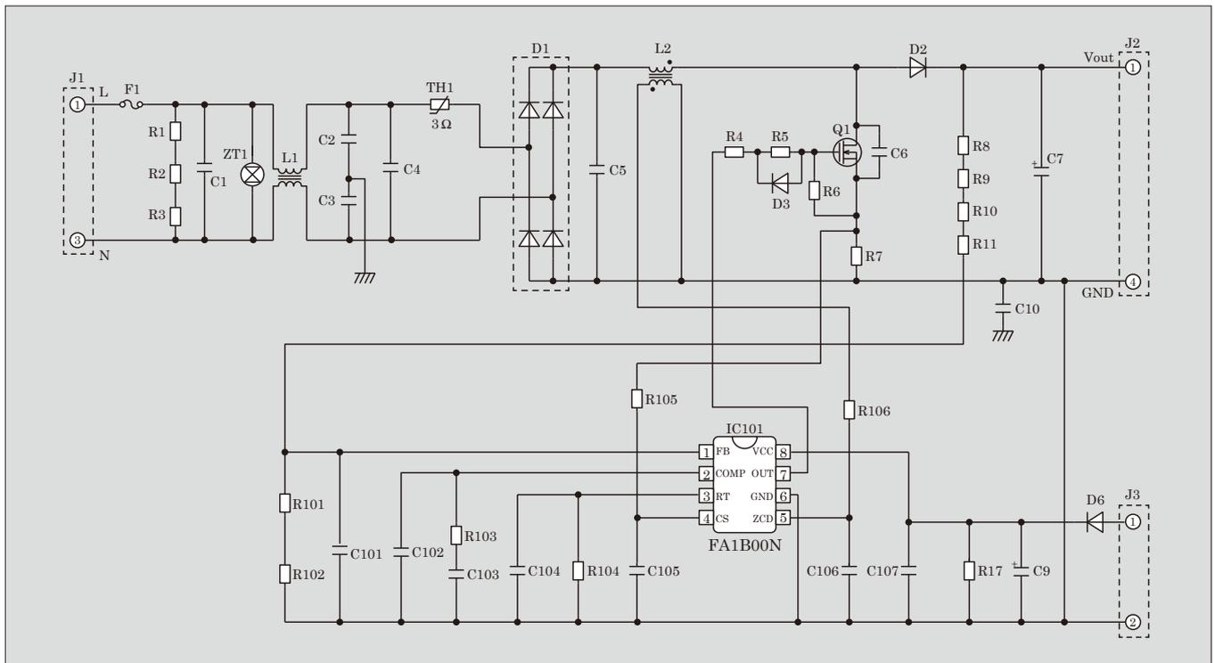
Fig.8 Application circuit example
