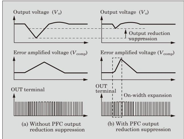
Fig.6 PFC output reduction suppressing function operation waveform
