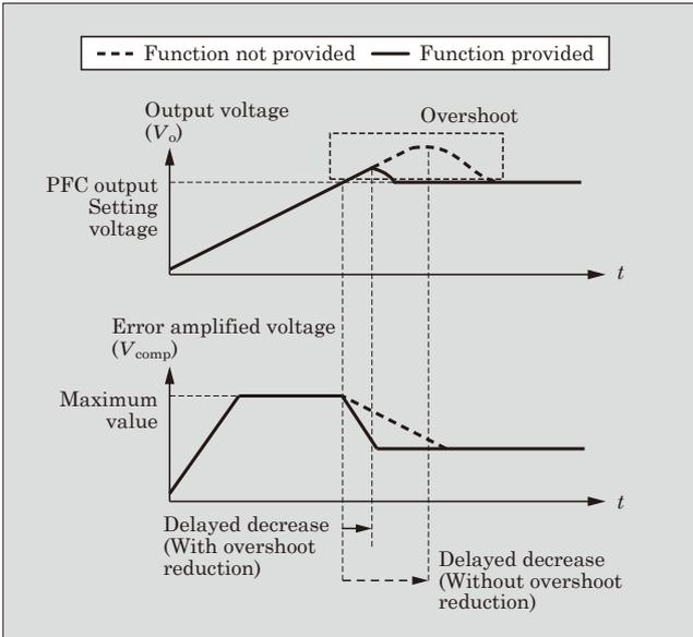
Fig.5 Overshoot reduction function operation waveform
