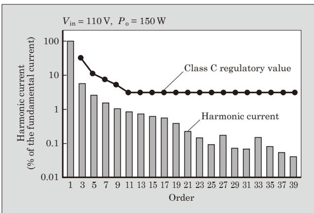
Fig.10 Harmonic current characteristics
