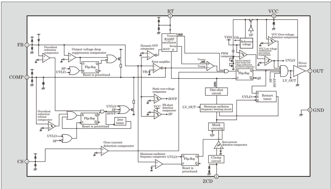
Fig.2 "FA1B00N" block diagram
