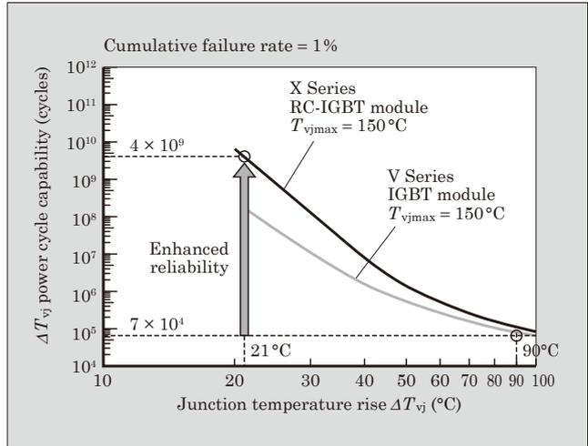
Fig.6  $\Delta T_{vj}$  power cycle capability
