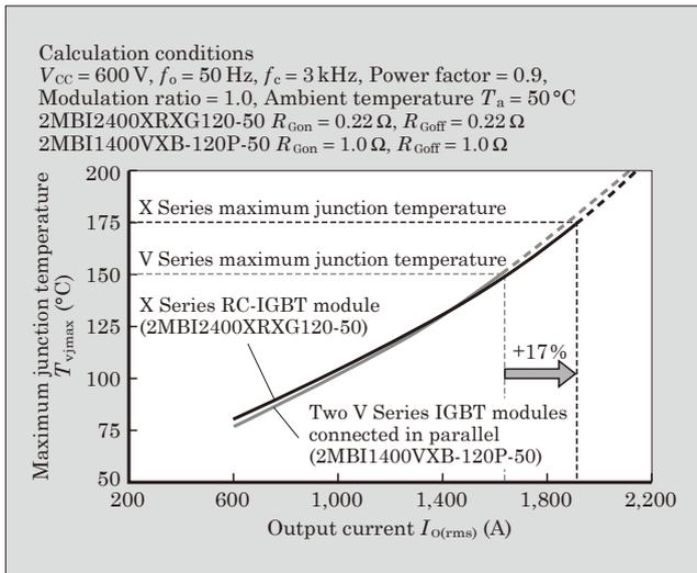
Fig.10 Maximum junction temperature at continuous operation
