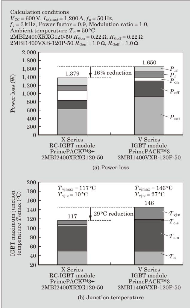
Fig.4 Power loss and junction temperature
