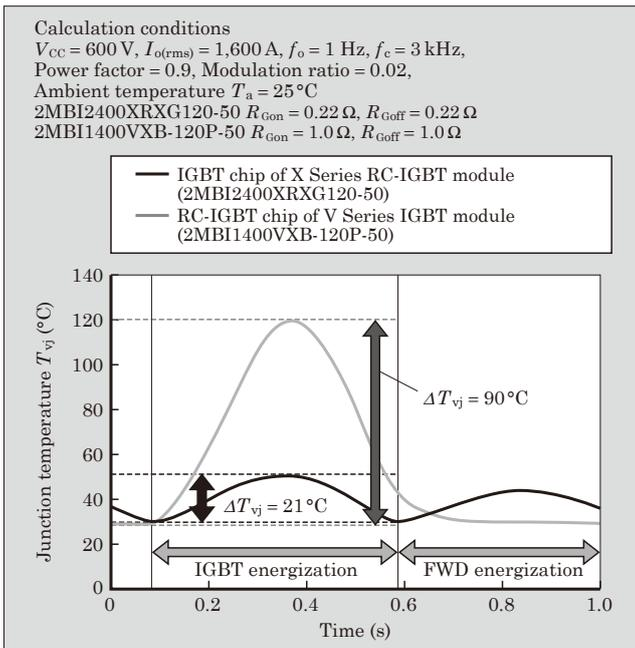
Fig.5 Low-frequency operation junction temperature  $T_{vj}$  time fluctuation
