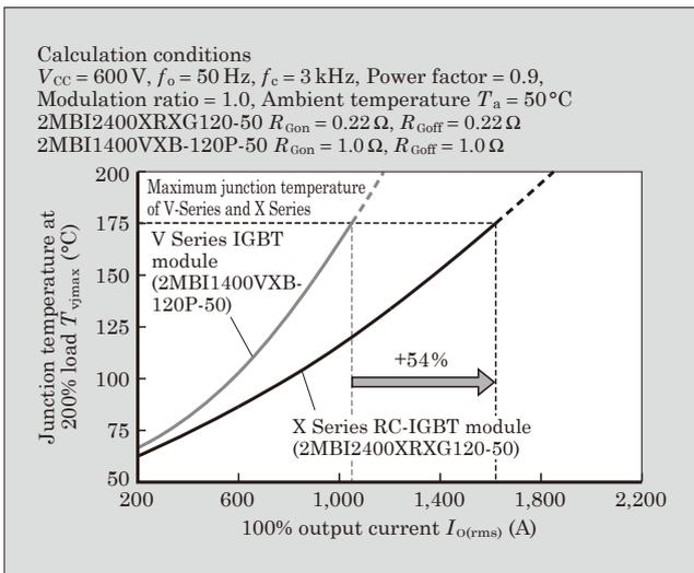
Fig.9 Maximum junction temperature at overloaded operation
