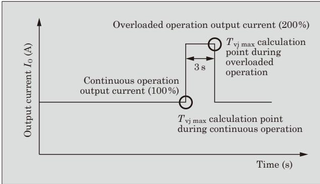
Fig.8 Operation pattern when overloading inverter overload
