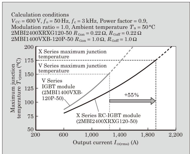
Fig.7 Maximum junction temperature at continuous operation
