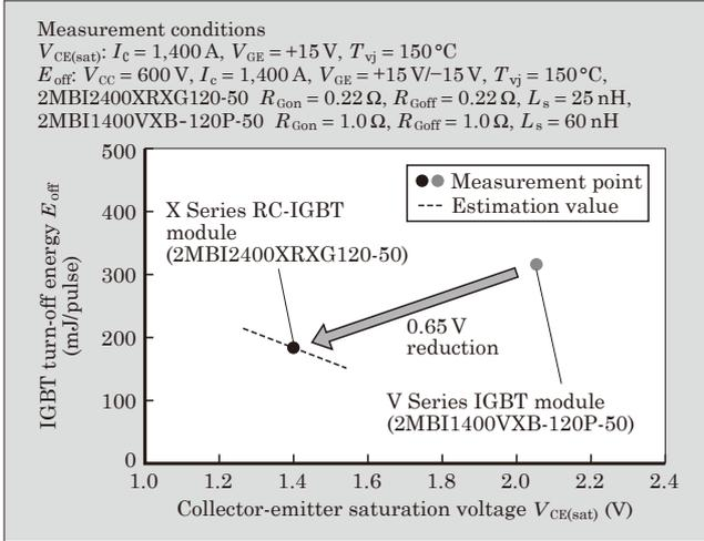
Fig.2 IGBT trade-off characteristics
