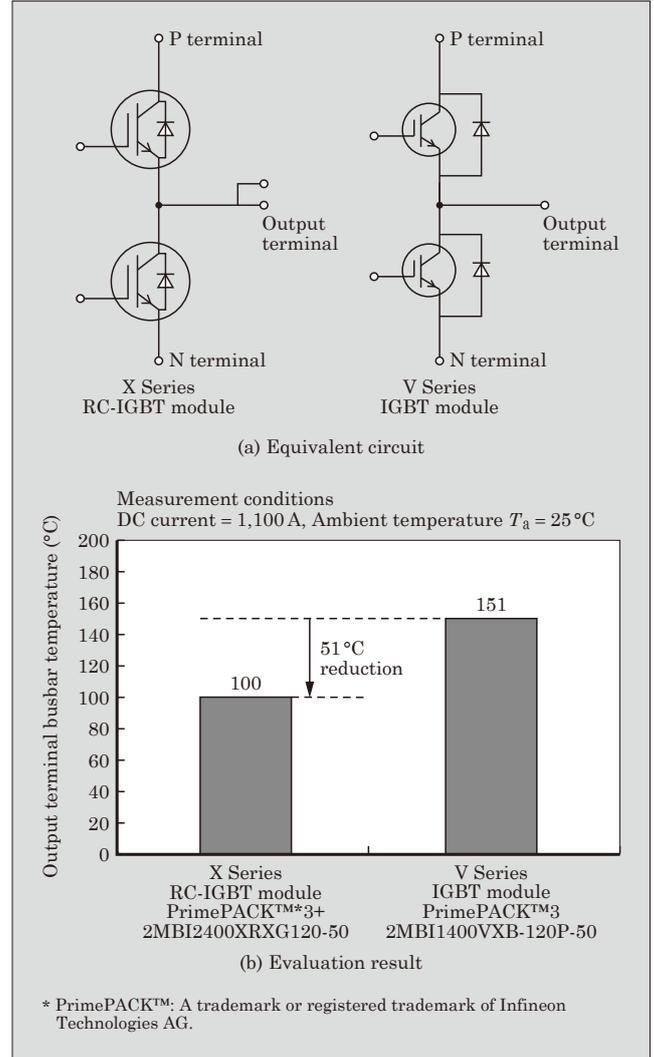
Fig.3 Equivalent circuit and terminal temperature evaluation results
