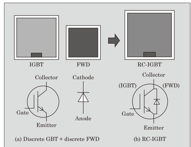
Fig.1 Schematic diagram and equivalent circuit of the 7th-generation X Series RC-IGBT for industrial applications
