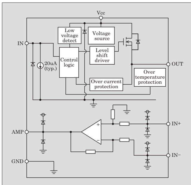
Fig.3 Circuit block diagram of “F5202H”
