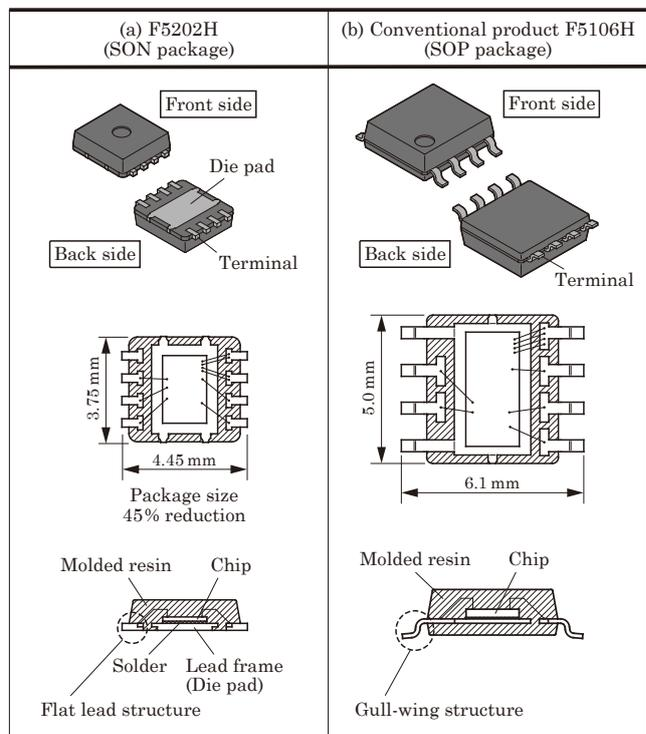
Fig.2 Comparison of package appearance and internal structure
