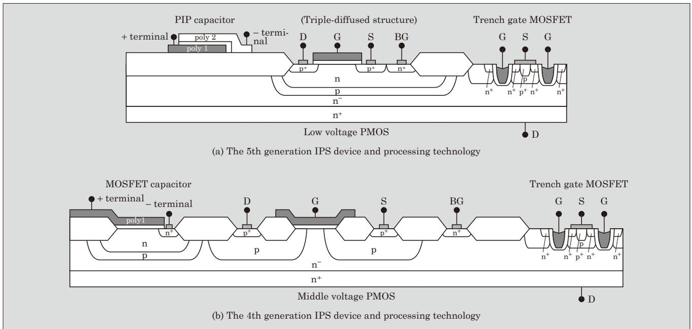
Fig.5 Comparison of key device and processing technologies for operational amplifiers and output stages
