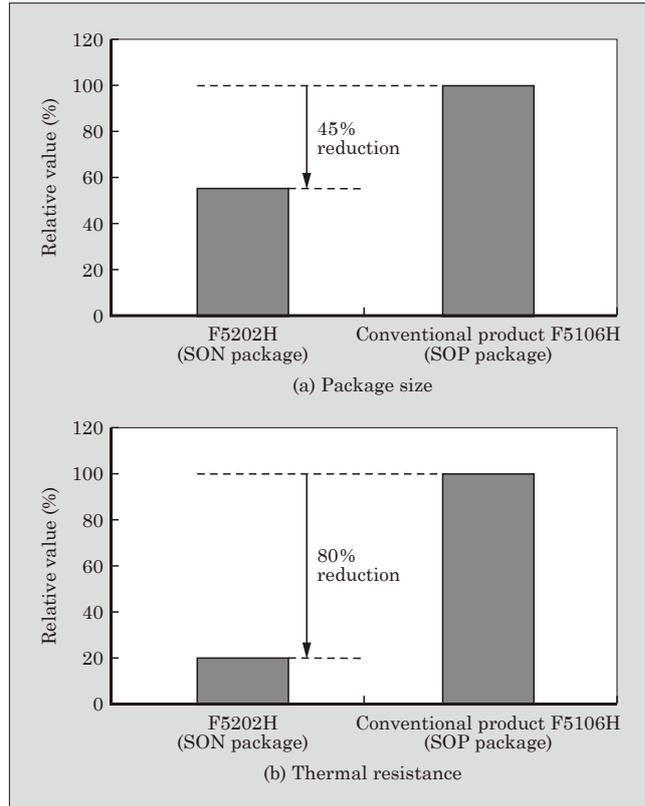
Fig.6 Comparison of SON package and conventional SOP package
