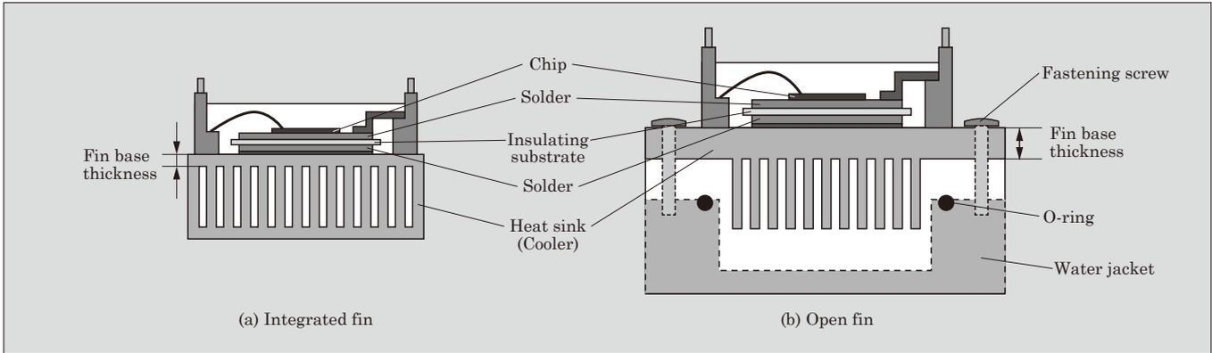
Fig.2 Cross-sectional view of integrated fin and open fin
