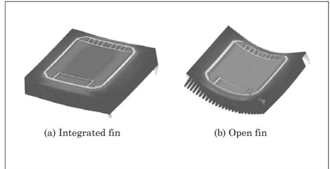
Fig. 7 Thermal stress simulation of elemental models of integrated fin and open fin
