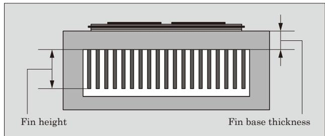
Fig.4 Cross-sectional view of the cooler
