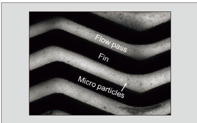
Fig.13 Measurement of particle motion in a cooler channel using PIV
