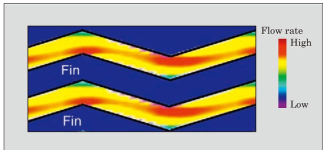
Fig.12 Calculation results of the velocity distribution in the cooler channel obtained through computational thermo-fluid simulation
