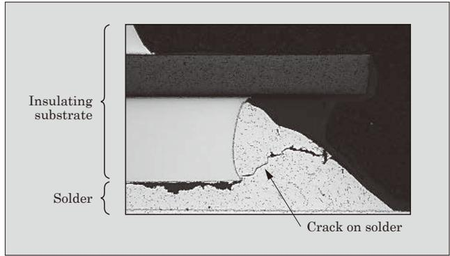
Fig.11 Fracture condition of solder joint under insulating substrate after thermal cycle test
