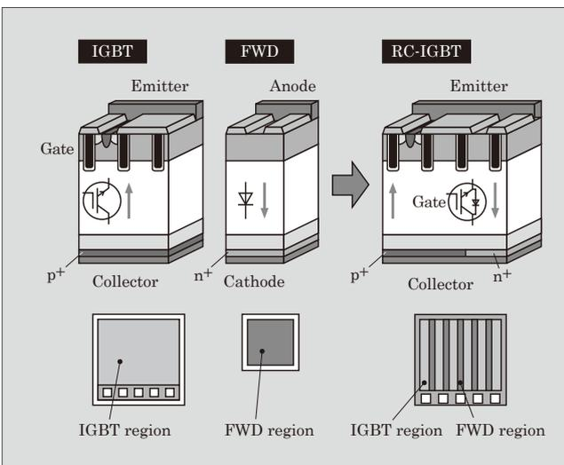
Fig.4 Comparison between separate chips and RC-IGBT
