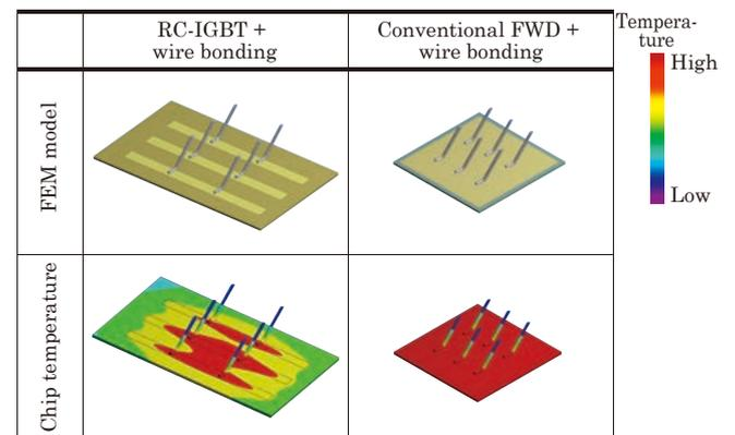
Fig.6 Thermal simulation of wire bonding structure
