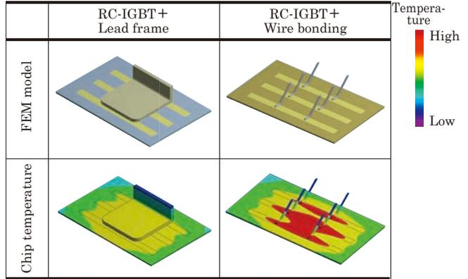
Fig.8 Thermal simulation of LF and wire bonding structures
