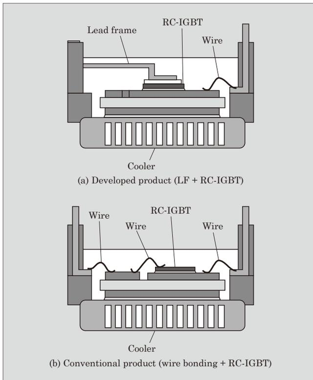
Fig.7 Structure comparison between developed and conventional products
