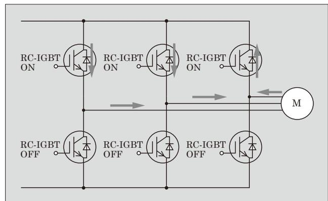
Fig.2 Example of current route in active short circuit (ASC)
