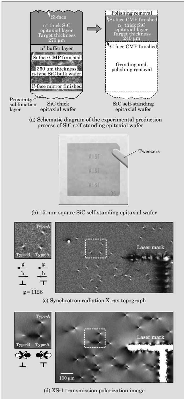
Fig.3 Evaluation of dislocations by using SiC self-standing epitaxial wafer
