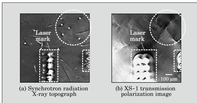
Fig.2 Example of comparative evaluation n-type SiC bulk wafer
