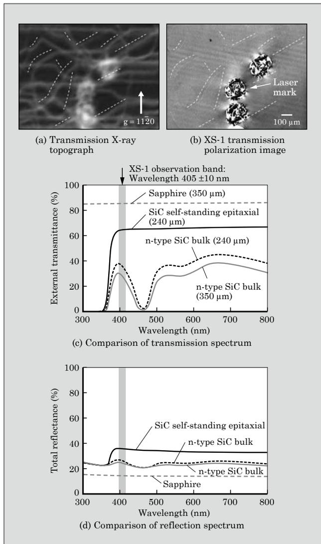
Fig.4 Evaluation of basal plane dislocation(BPD) by using sapphire wafer
