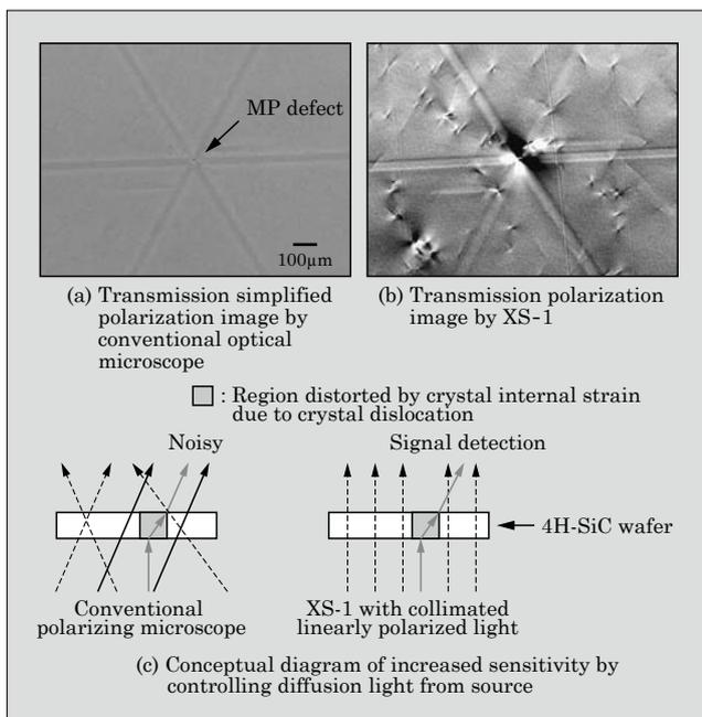
Fig.1 Effect of diffusion light from source in transmission polarization observation
