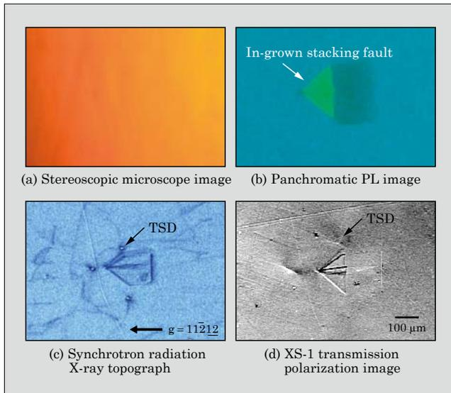
Fig.5 Evaluation example of stacking faults in SiC epitaxial film by transmission polarization image
