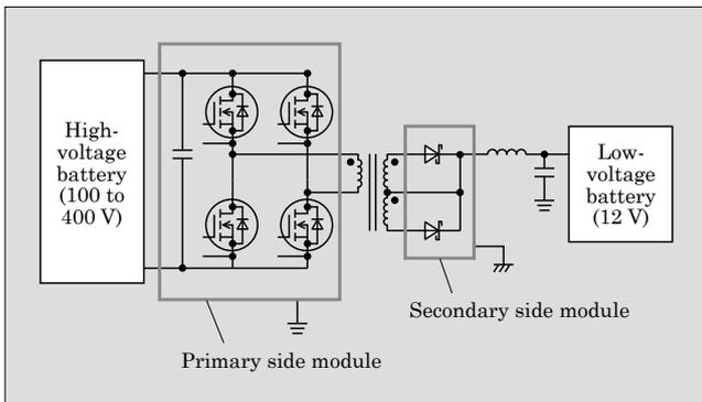
Fig.3 Equivalent circuit diagram of the DC-DC converter module
