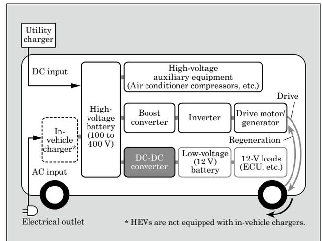
Fig.1 xEV block diagram
