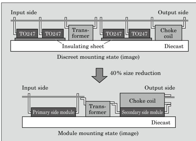
Fig.8 Footprint ratio of a DC-DC converter system
