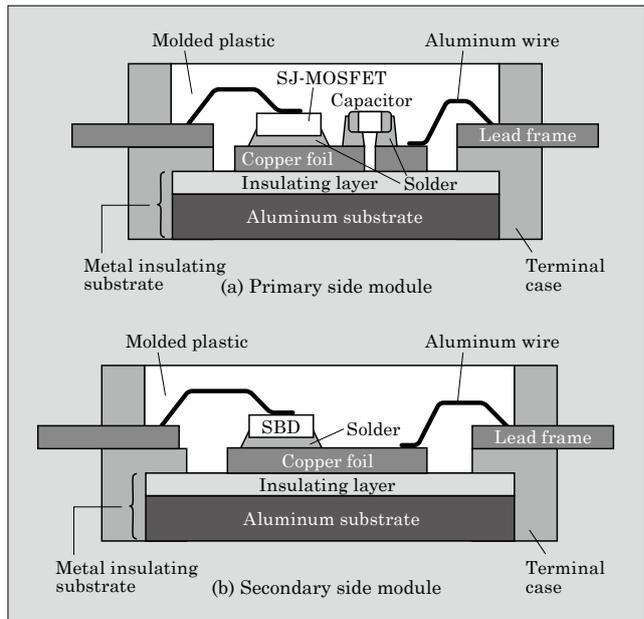
Fig.4 Cross-sectional structure of the DC-DC converter module
