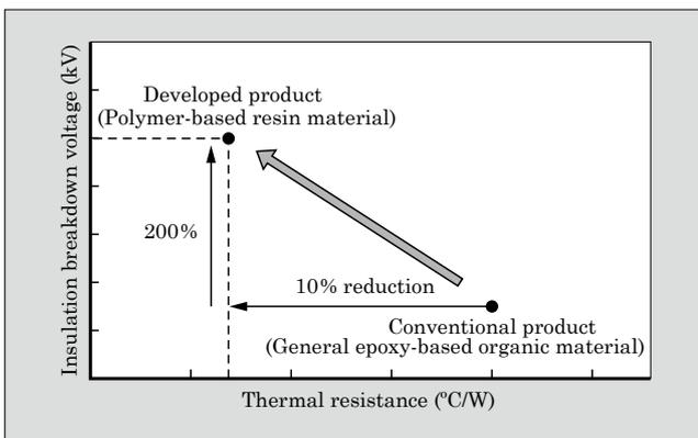
Fig.5 Comparison of insulating layers
