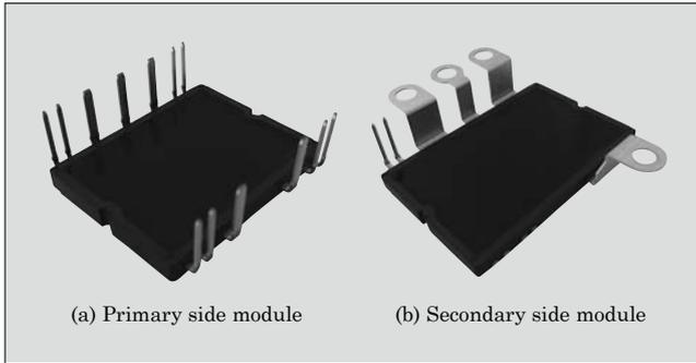
Fig.2 DC-DC converter modules
