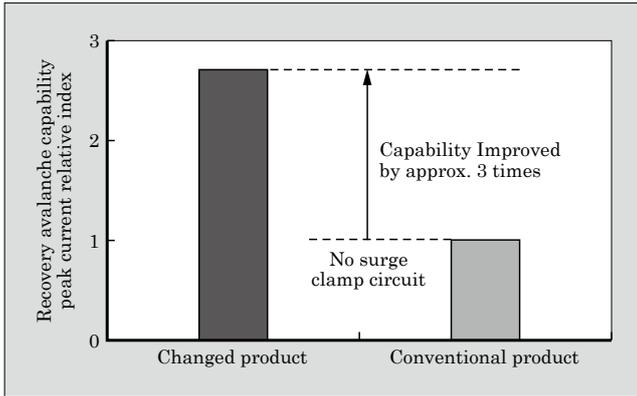
Fig.7 Comparison of surge voltage tolerance
