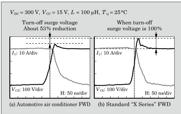
Fig.6 Switching waveform at turn-off
