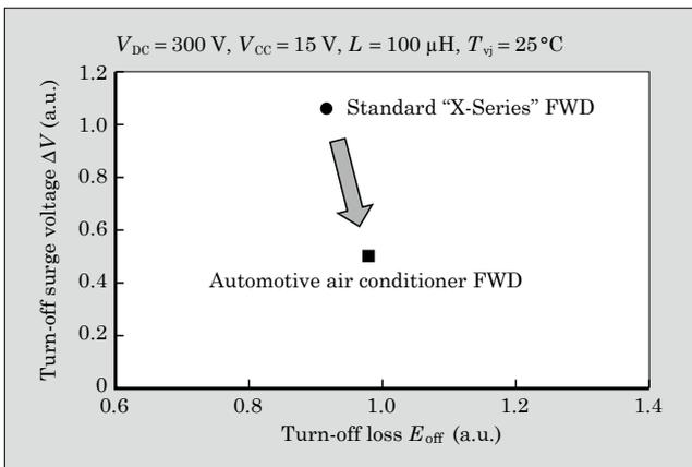
Fig.7 Turn-off surge voltage and turn-off loss trade-off characteristic
