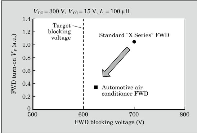
Fig.5  $V_F$  and blocking voltage characteristic at FWD turn-on
