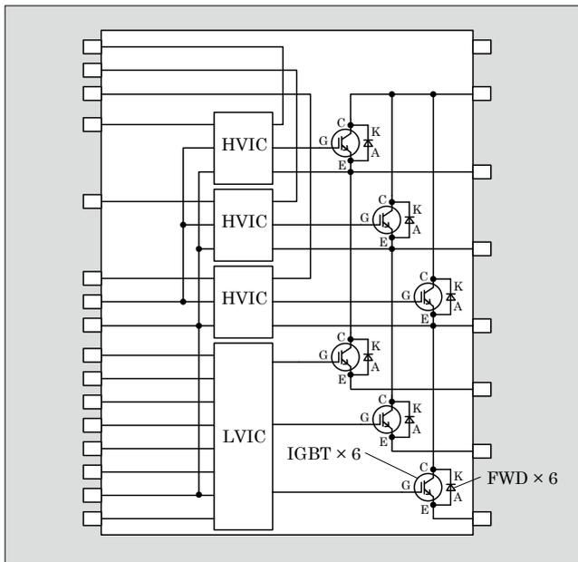
Fig.2 Internal equivalent circuit
