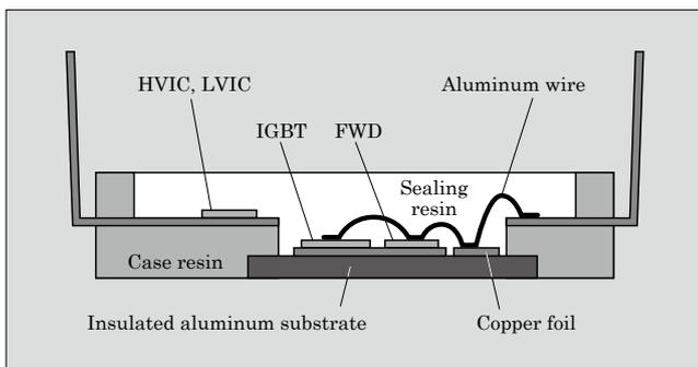
Fig.3 Package cross-sectional structure
