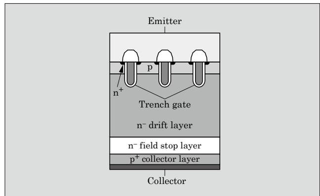
Fig.4 "X-Series" IGBT chip cross-sectional structure
