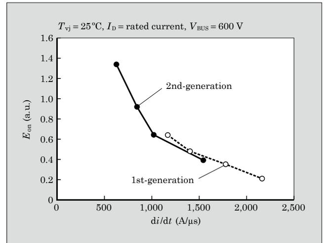
Fig.8 Comparison of turn-on loss
