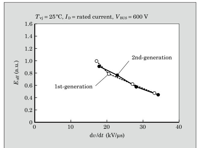
Fig.9 Comparison of turn-off loss
