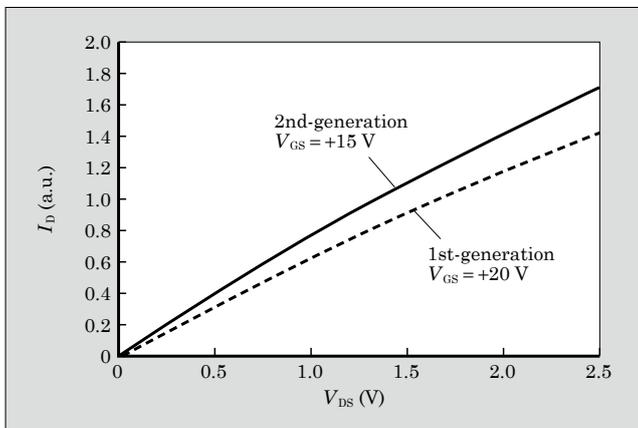
Fig.2 1st-generation and 2nd-generation SiC trench-gate MOSFET  $I_D$ - $V_{DS}$  characteristic (first quadrant)
