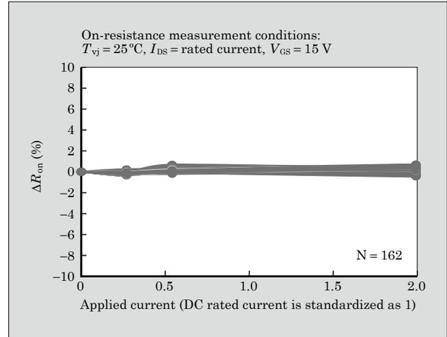
Fig.12 Fluctuation rate of on-resistance after body diode conduction test (Application conditions:  $T_{vj} = 175^\circ\text{C}$ ,  $V_{GS} = -3\text{ V}$ , Time = 10 min)
