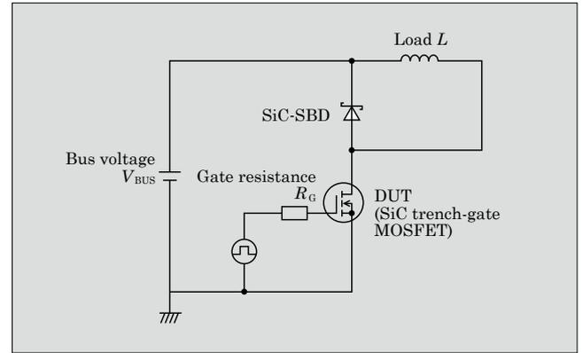
Fig.7 Switching evaluation circuit
