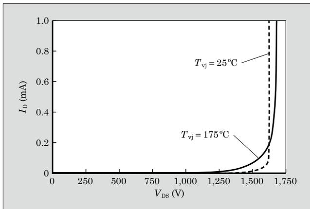
Fig.6  $I_D$ - $V_{DS}$  characteristic during 2nd-generation SiC trench-gate MOSFET off-state
