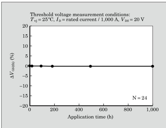
Fig.11 Fluctuation rate of threshold voltage after high-temperature gate negative bias test (Application conditions:  $T_{vj} = 175^\circ\text{C}$ ,  $V_{GS} = -7\text{ V}$ )
