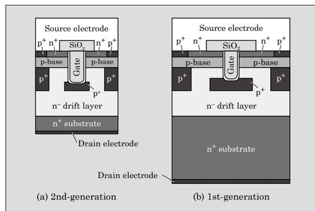
Fig.1 Structure of 1st-generation and 2nd-generation SiC trench-gate MOSFETs
