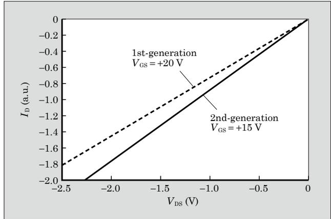
Fig.3 1st-generation and 2nd-generation SiC trench-gate MOSFET  $I_D$ - $V_{DS}$  characteristic (third quadrant)
