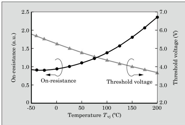
Fig.5 Temperature dependence of on-resistance and threshold voltage of 2nd-generation SiC trench-gate MOSFETs
