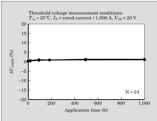
Fig.10 Fluctuation rate of threshold voltage after high-temperature gate positive bias test (Application conditions:  $T_{vj} = 175^\circ\text{C}$ ,  $V_{GS} = 20\text{ V}$ )
