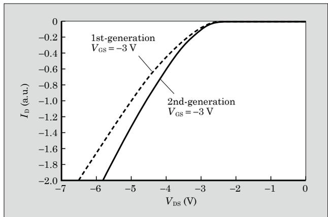
Fig.4 1st-generation and 2nd-generation SiC trench-gate MOSFET body diode  $I_D$ - $V_{DS}$  characteristic (third quadrant)
