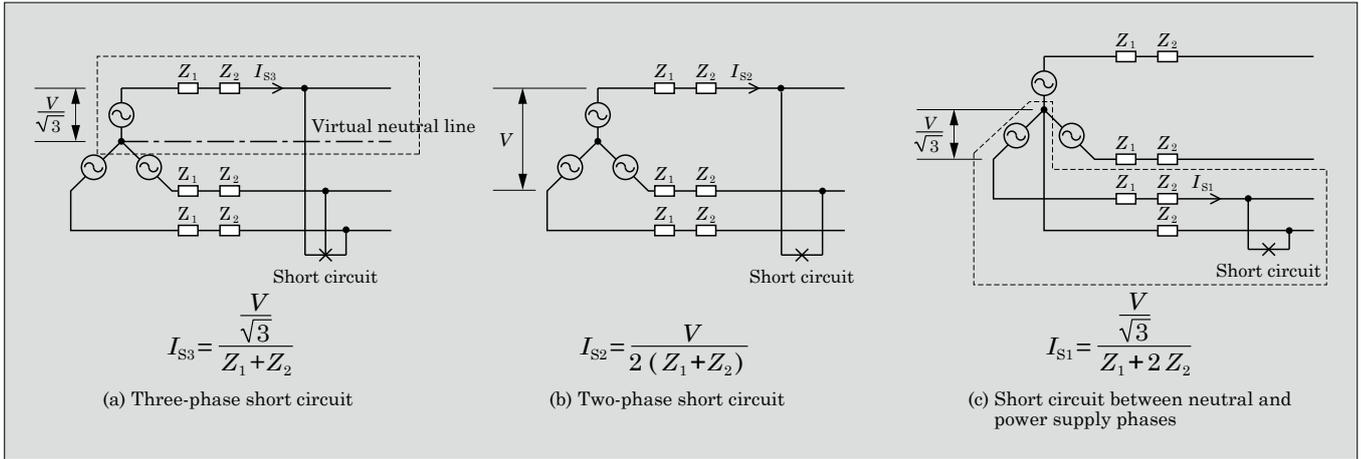
Fig.5 Short-circuit current calculation equation for three-phase short circuit, two-phase short circuit and short circuit between neutral and power supply phases
