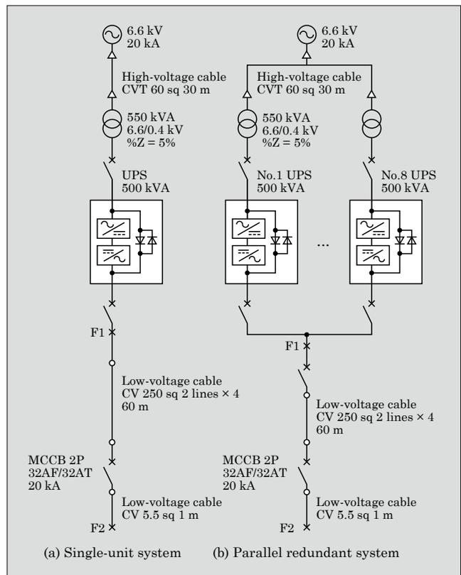
Fig.4 Impedance maps of single-unit and parallel redundant systems
