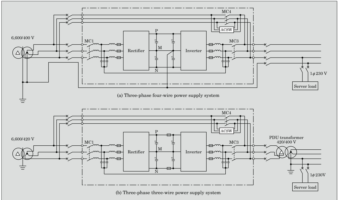
Fig.1 Main circuit wiring diagrams of three-phase, four-wire and three-phase, three-wire power supply systems
