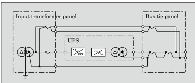
Fig.3 Three-phase, four-wire power supply system using “UPS6000DX” (three-phase, three-wire)
