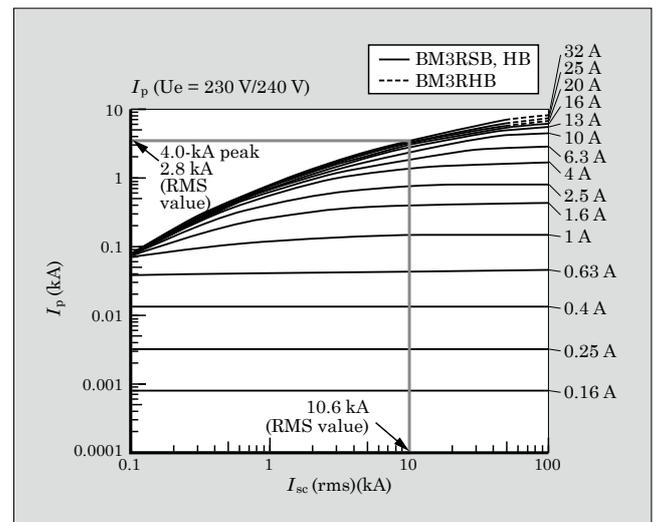
Fig.6 Cutoff characteristic of “BM Series” current-limiting circuit breakers
