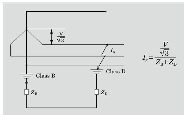
Fig.7 Ground-fault current equivalent circuit and calculation equation
