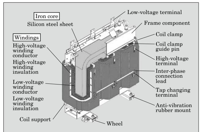
Fig.5 Structure of molded transformer
