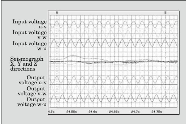
Fig.3 Input voltage and output voltage waveforms during vibration
