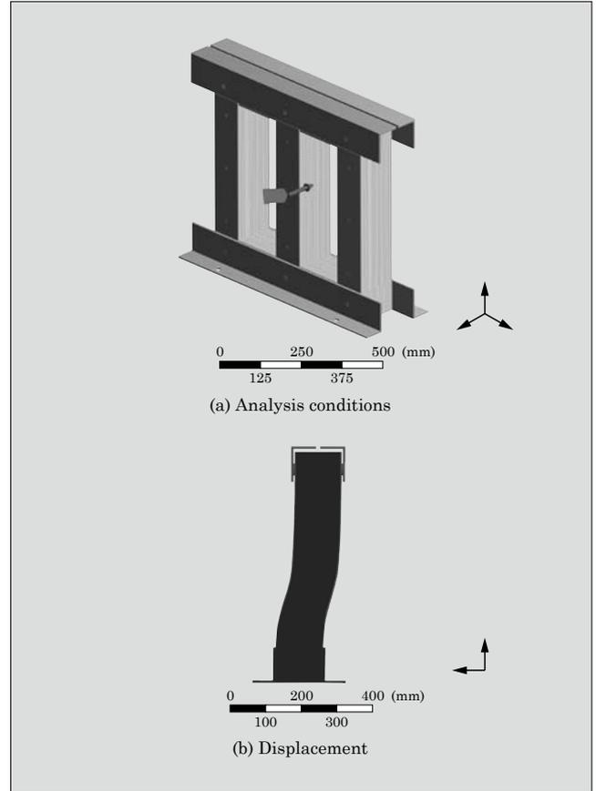
Fig.4 Results of static analysis of transformer
