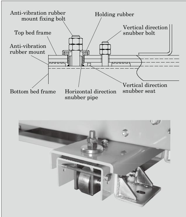
Fig.6 Structure of seismic snubber of molded transformer
