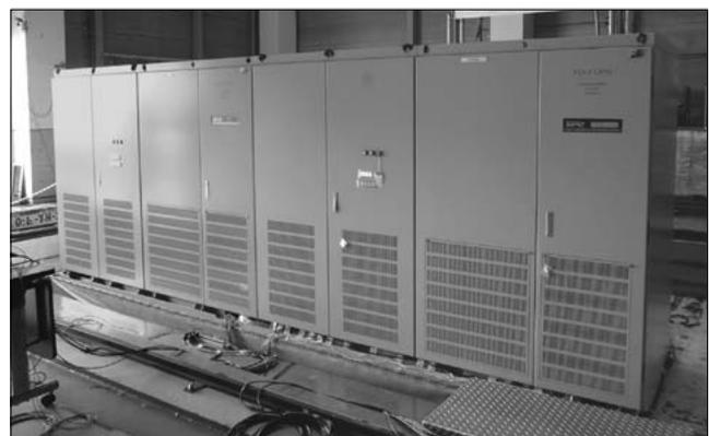
Fig.2 UPS equipment installed on vibration table
