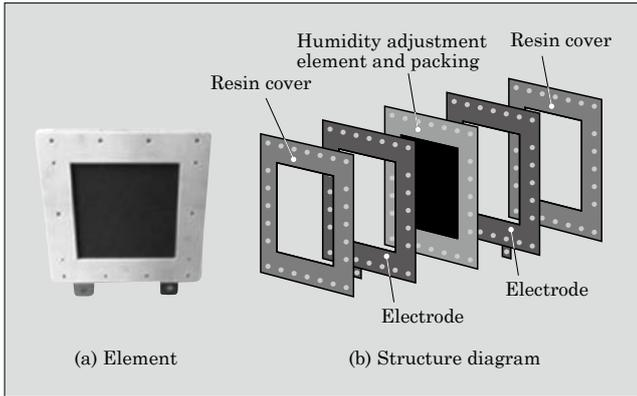
Fig.2 External appearance and structure of the element
