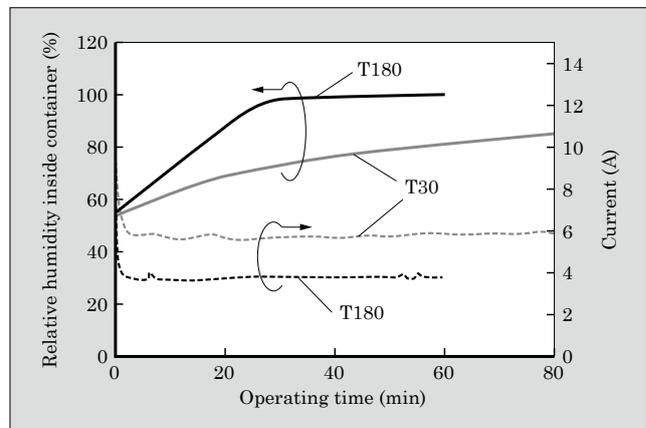
Fig.4 Transition result of humidifying amount and electric current
