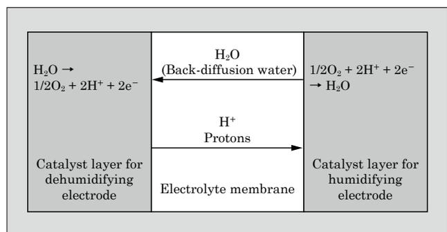
Fig.5 Schematic diagram of water movement in the element
