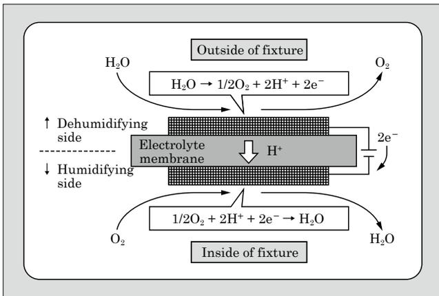
Fig.3 Reaction schematic diagram
