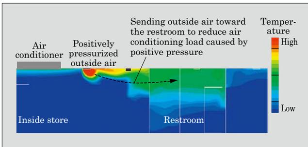
Fig.11 In-store temperature distribution at time of outside air intrusion
