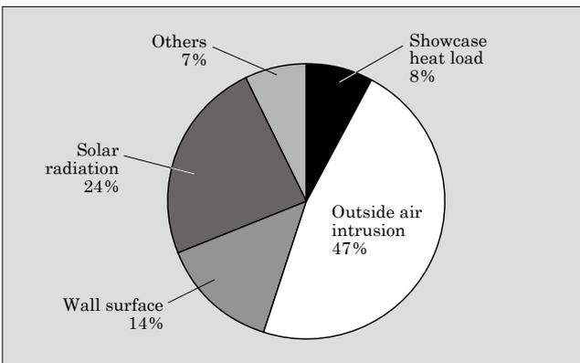
Fig.8 Heat load factor analysis results for air conditioning system
