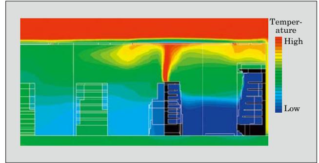
Fig.5 Temperature distribution based on heat and airflow analysis
