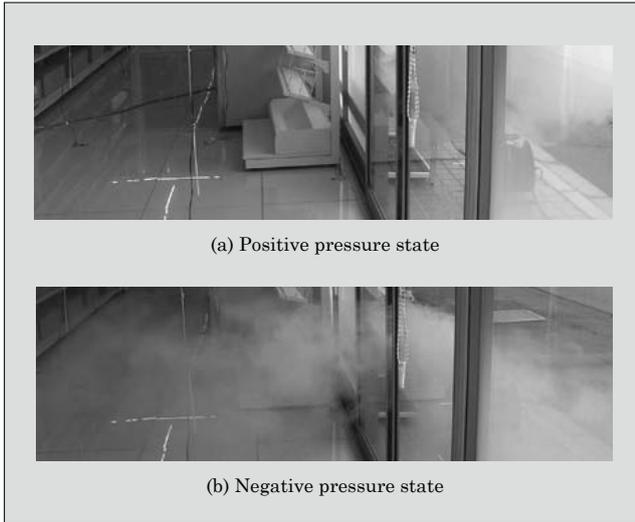
Fig.10 Effect of reducing intrusion of outside air from doors
