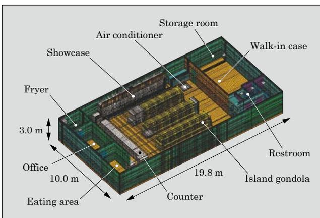
Fig.4 Heat and airflow analysis model
