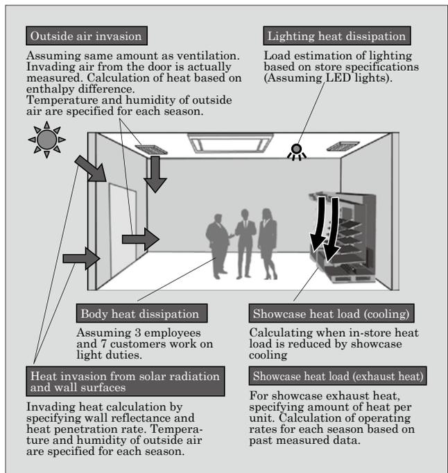
Fig.2 Parameters considered by the heat balance calculating unit
