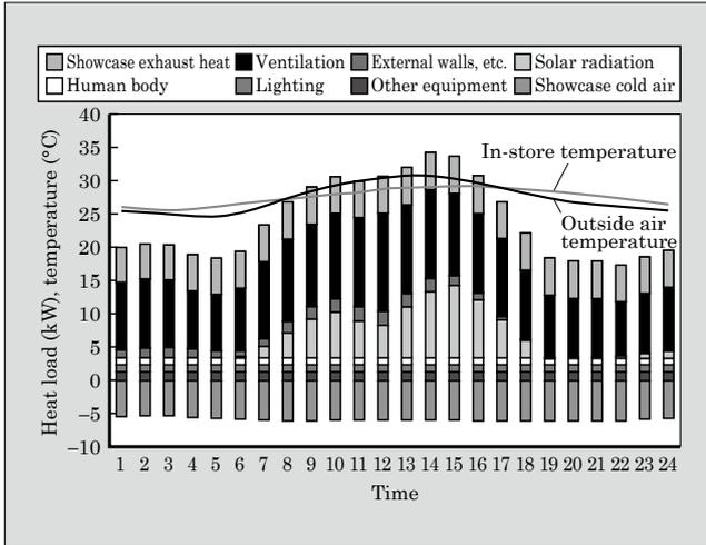
Fig.3 Heat balance calculation results
