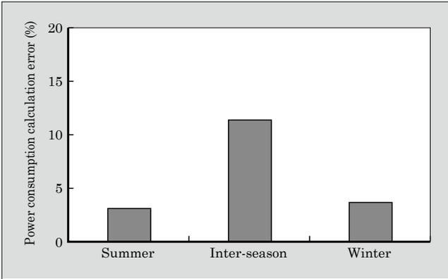
Fig.7 Calculation error in power consumption calculated with the in-store heat balance analysis tool
