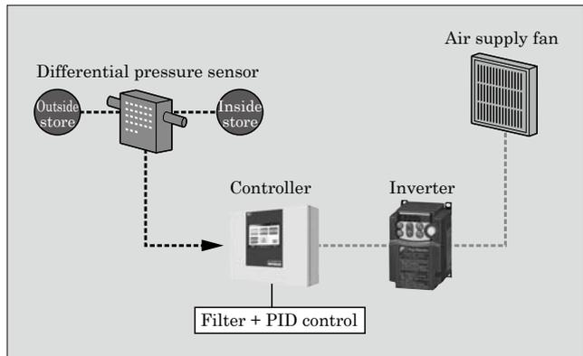
Fig.9 Positive pressure control system
