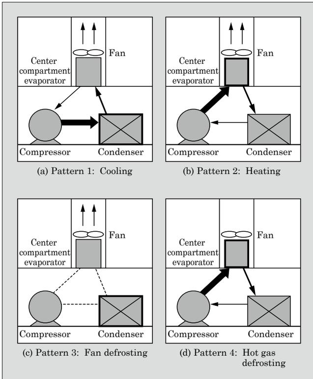
Fig.3 Refrigerant passage in each operation mode
