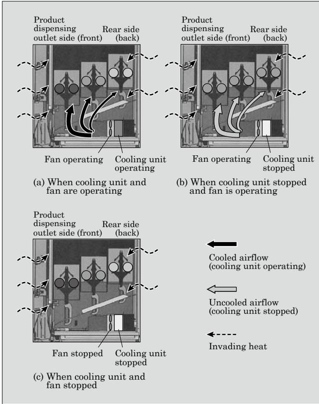
Fig.7 Cross-sectional view of inside of center compartment during cooling operation
