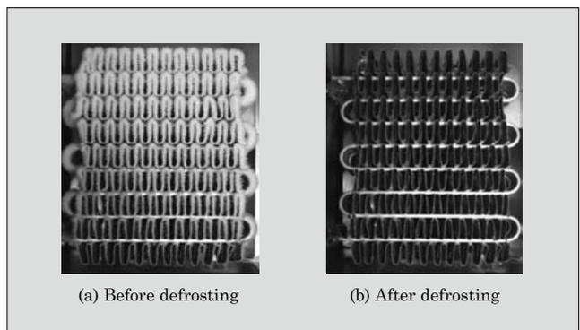
Fig.4 Evaporator before and after hot-gas defrosting of developed machine
