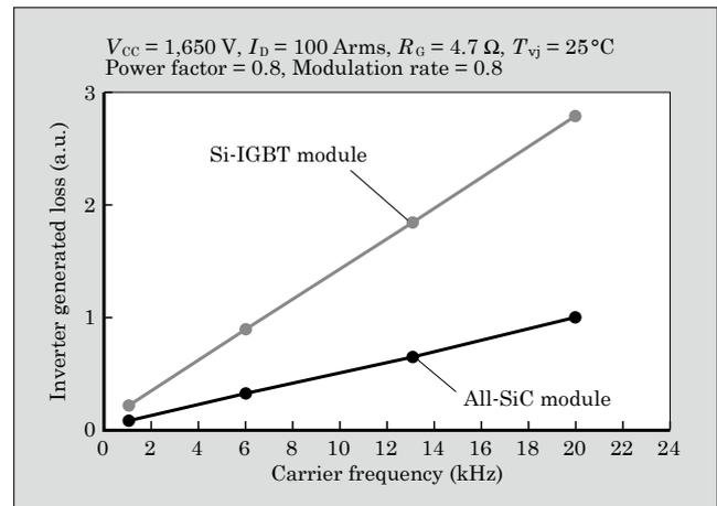
Fig.12 Carrier frequency dependence of inverter generated loss
