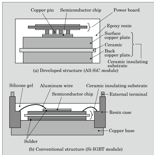
Fig.3 Comparison of modules' cross-sectional schematic structures
