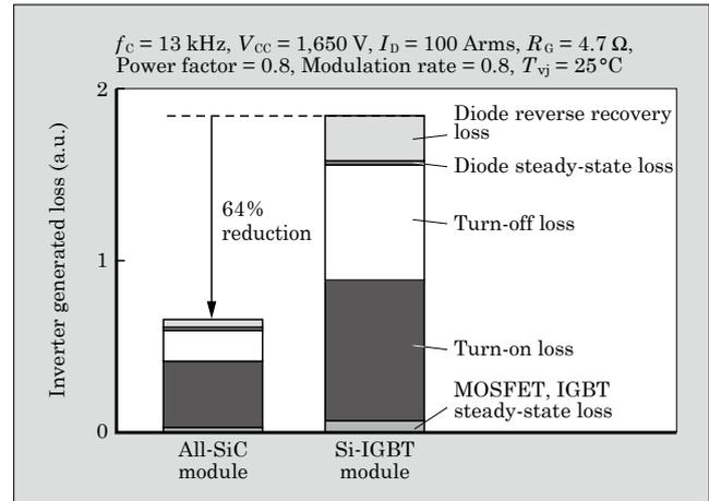
Fig.11 Inverter generated loss simulation
