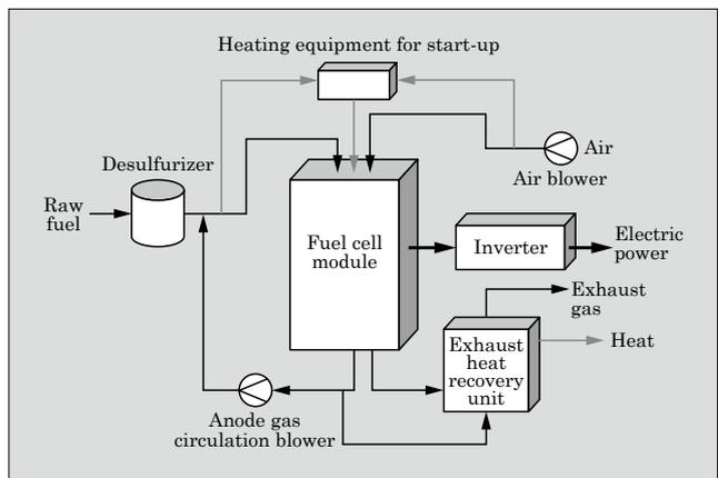
Fig.8 Equipment configuration of SOFC
