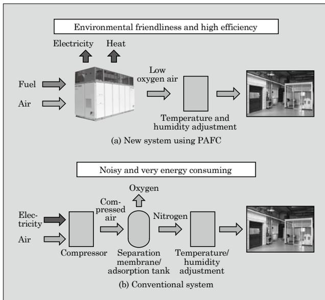
Fig.4 Comparison of systems that reduce oxygen concentration indoors
