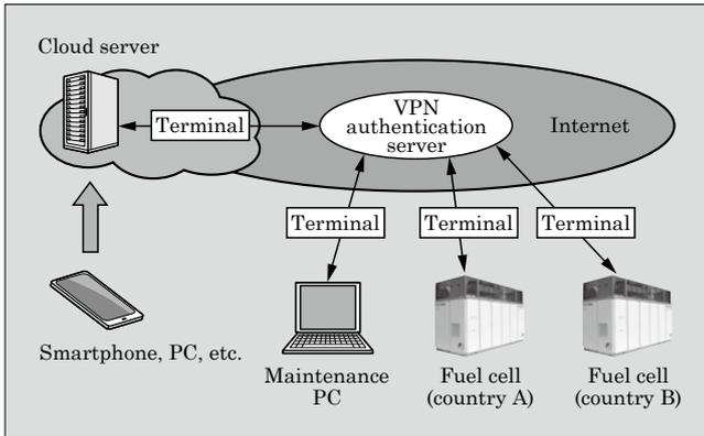
Fig.6 Cloud-based fuel cell remote monitoring system and maintenance system
