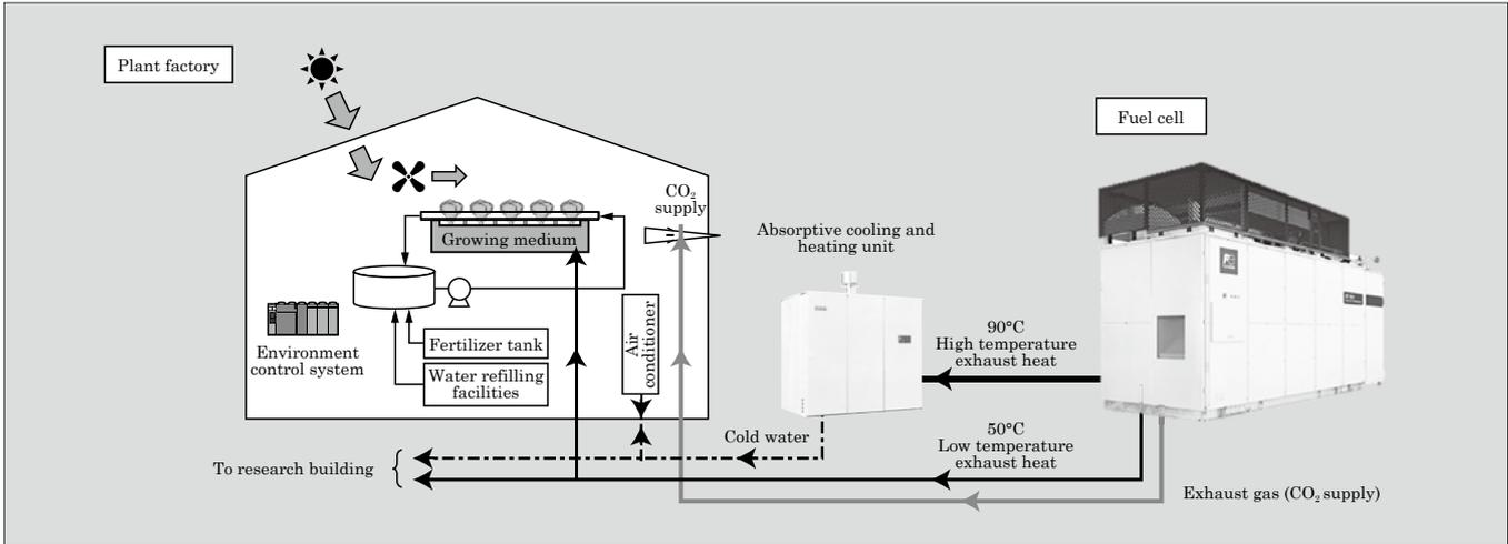
Fig.2 Cogeneration system and supply of CO<sub>2</sub> to plant factory inside Tokyo Factory
