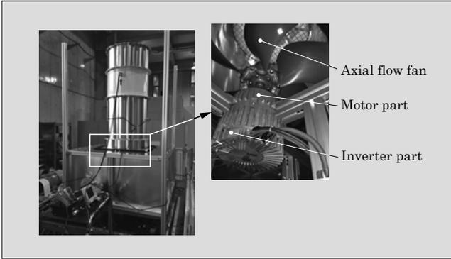
Fig.5 Actual load test device
