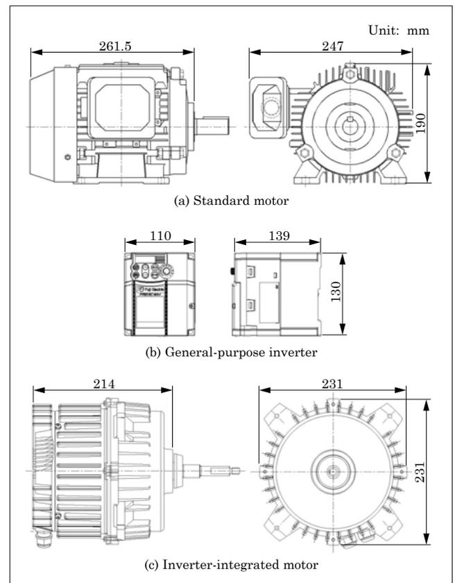
Fig.11 Dimensions of each model
