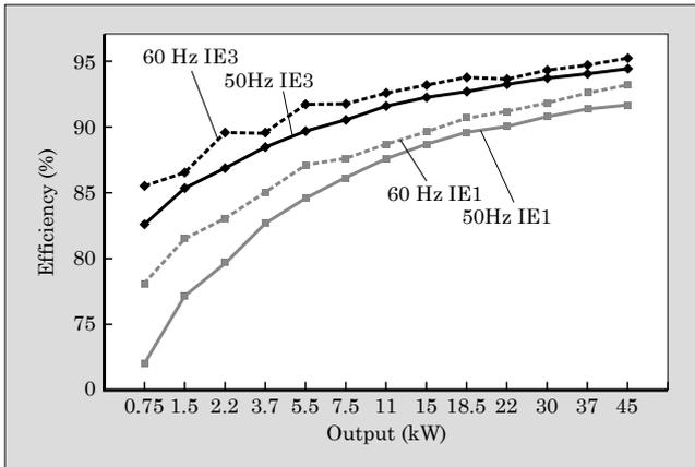
Fig.2 Efficiency comparison among Fuji Electric's representative types
