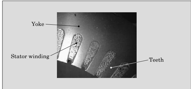
Fig.5 Cross section of stator iron core (part)
