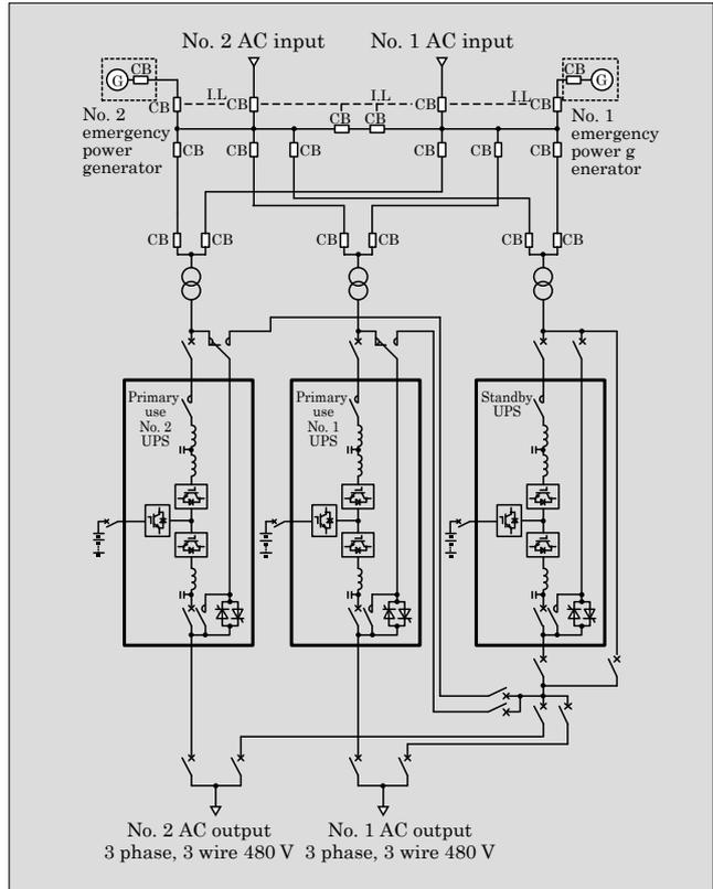
Fig.3 System configuration of standby redundant operation system
