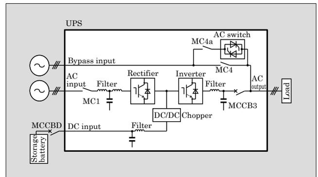
Fig.5 Main circuit block diagram
