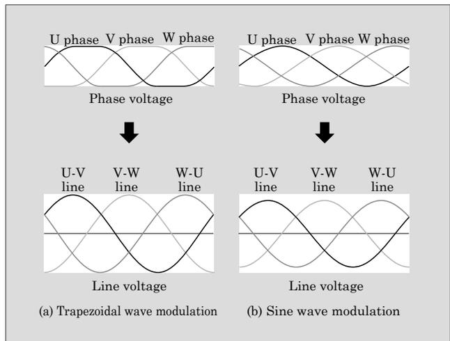
Fig.9 Voltage waveform of rectifier and inverter
