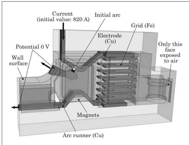
Fig.11 Arc analysis model for molded-case circuit-breakers
