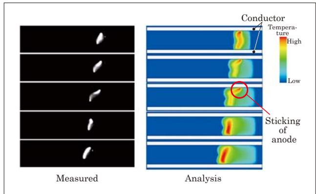
Fig.3 Inchworm movement of arc on parallel conductors
