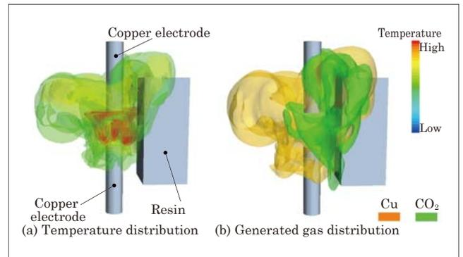
Fig.7 Example of arc simulation by electrodes butting
