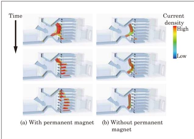
Fig.14 Simulation results at the time of interruption of 100 A
