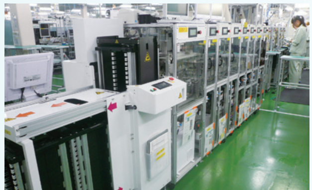
Automated printed circuit board inspection line
