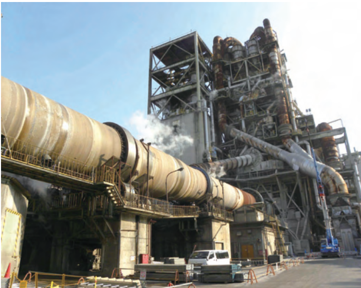
The cylinder in the foreground at the Saitama Plant of Taiheiyo Cement Corporation is a cement incineration kiln
