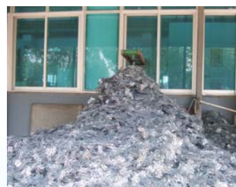
Punch plate generated during the press process
