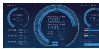
Our EMS reduces environmental loads through "visualization" via real-time measurement of energy usage, "clarification" through analysis of operation statuses, and "optimization" by optimizing the operation of entire facilities.
