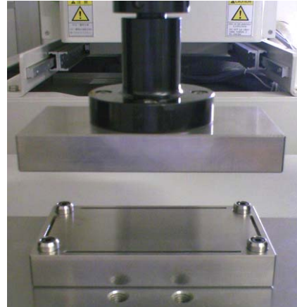
2 Place PCB on the lower tool to fit the PCB-guides.
