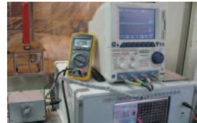
Partial discharge measurement
