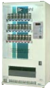
Fuji Electric, in cooperation with Tokyo Electric Power Co., Inc. and Coca-Cola Japan Co., Ltd., has developed a new vending machine designed to ease the peak summertime demand for electricity by chilling beverages at off-peak times and shutting down the refrigeration unit during times of peak demand.
