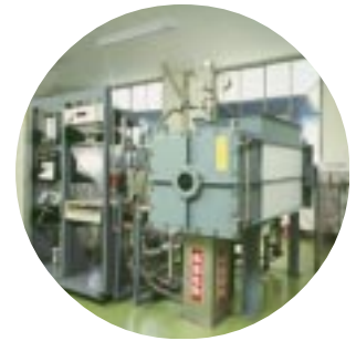
We developed a high-concentration ozone generator for advanced ozone water and sewage purification systems.
