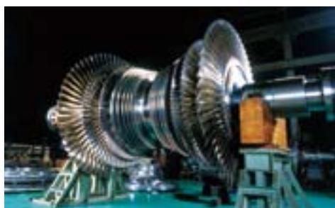
Materials specially suited to resist the corrosive components contained in geothermal steam are used in turbines for geothermal power generation.
