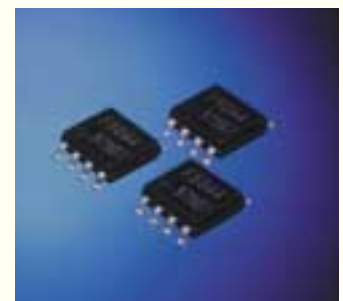
The Smart MOSFET responds to the demand for small, lightweight electronic control devices for automotive applications.
