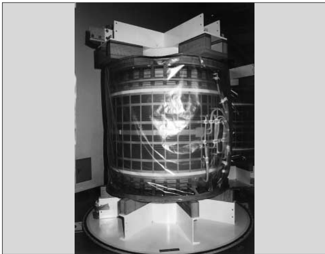
Fig.3 Winding assembly packaged with film
