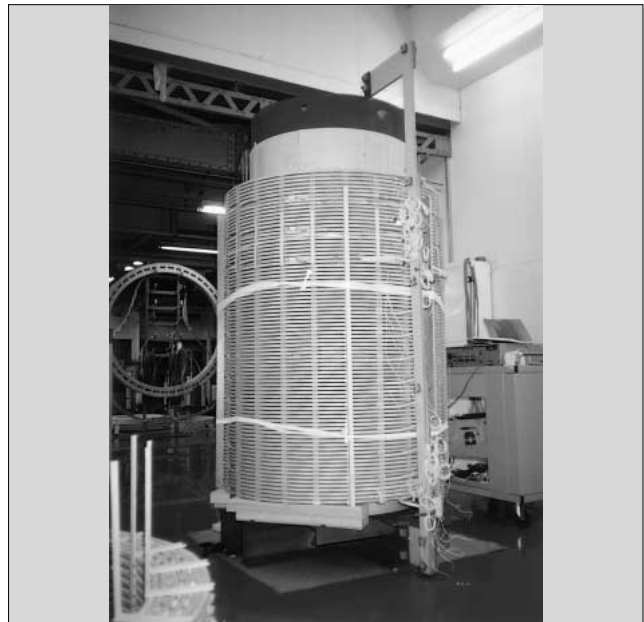
Fig.2 Actual-scale model of interleaved disc winding using transposed conductors
