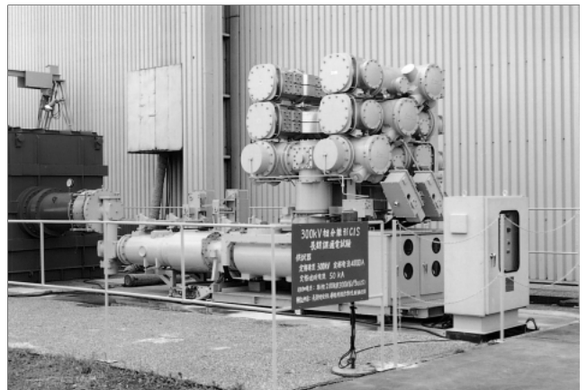
Fig.11 The state of long-term energizing test
