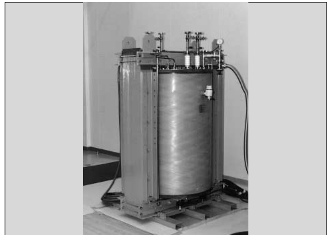
Fig.3 Liquid-nitrogen-cooled, single-phase, 500kVA superconducting transformer
