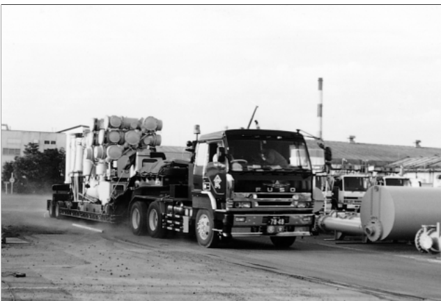
Fig.9 The state of transportation test
