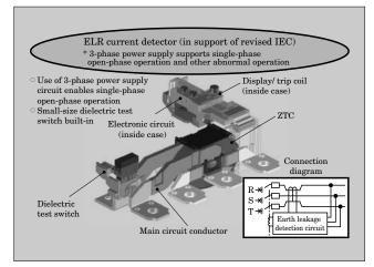
circuit tripped even in cases where one of the three phases is an open-phase. To support this requirement, a new small-size power supply circuit was developed and applied. In addition, ultra-miniaturization of the trip coil and modularization of mechanical parts that transfer motion enabled the successful development of a small-size earth leakage trip unit. (See Fig. 16.) As a result, the product was commercialized without having to modify the external dimensions of conventional products.
