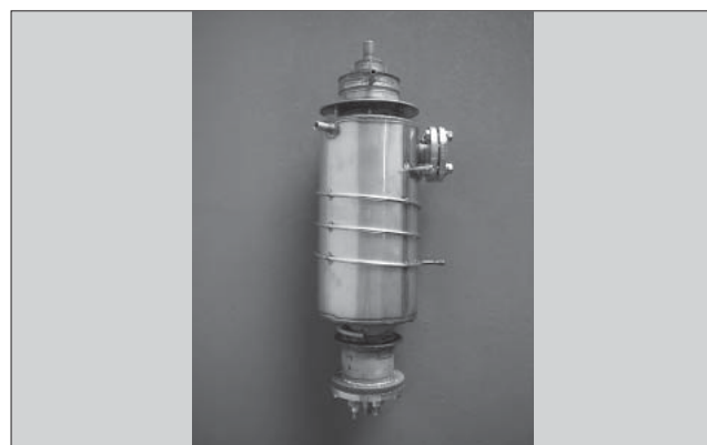
Fig.2 Appearance of the reformer/CO shift converter
