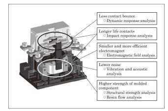
Fig.1 Simulation technology in contactor design
