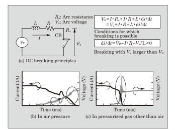
Fig.13 Basic study of high-voltage DC breaking
