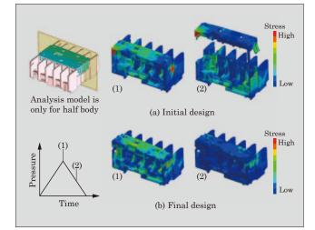
Fig.6 Stress analysis of miniature contactor terminal cover
