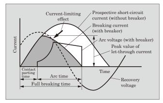
Fig.8 Current-limiting breaking characteristics for high breaking capacity
