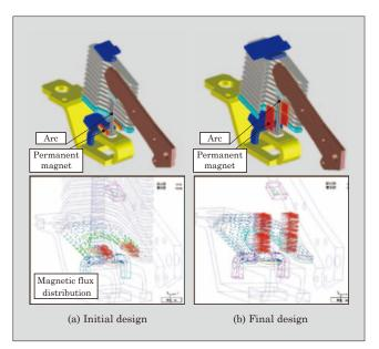
Fig.11 Electromagnetic analysis of MCCB cutoff part
