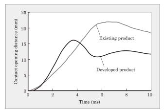
Fig.9 Comparison of contact opening characteristics
