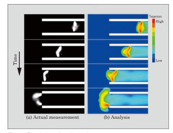
Fig.13 Simulation of arc behavior
