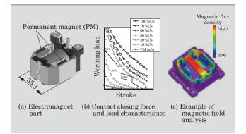
Fig.7 Miniaturization of electromagnet part of electromagnetic switch
