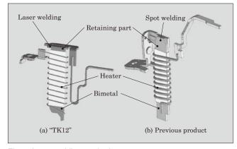
Fig.8 Laser welding method
