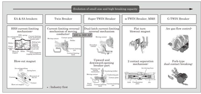
Fig.9 Technical development for higher breaking capacity of molded-case circuit breakers
