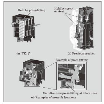
Fig.4 Example of press-fit parts
