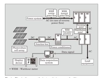
Fig.1 Block diagram of photovoltaic power facility
