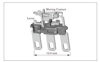
Fig.5 Example application to micro-actuator in command switch
