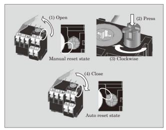
Fig.10 Automatic reset mode switching method
