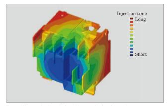
Fig.6 Example of molding flow analysis of housing
