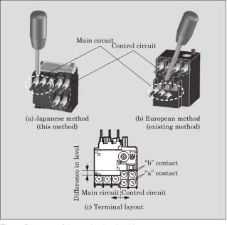
Fig.9 Diagram of the main circuit wiring
