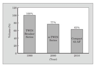
Fig.3 Miniaturization of low-voltage circuit breakers
