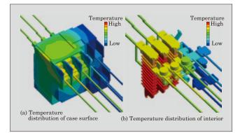
Fig.9 Thermal analysis of thermal relay
