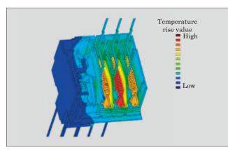
Fig.7 Coupled analysis example of current–electric heating– bimetal curvature
