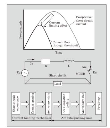
Fig.12 Current limiting breaking method
