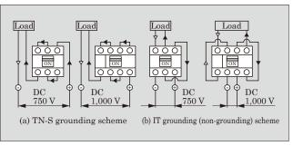
Fig.4 Grounding scheme and connection
