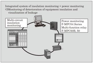
Fig.12 Power monitoring and insulation monitoring in the same system
