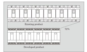
Fig.4 Miniaturization image on parallel installation
