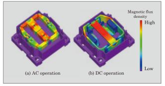
Fig.8 Magnetic field analysis
