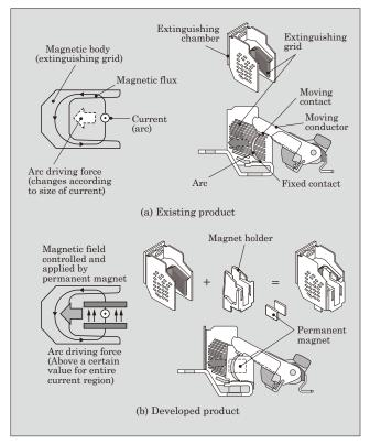
Fig.7 Basic structure of breaker
