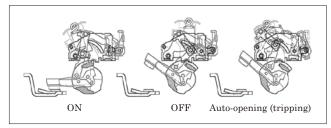
Fig.4 Example analysis of contact opening and closing mechanism used in molded-case circuit breakers
