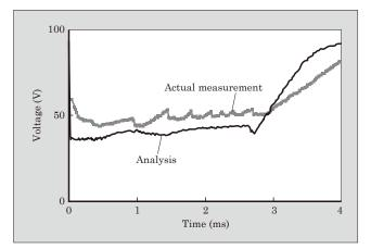
Fig.14 Comparison of arc voltage
