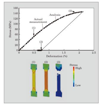
Fig.4 Simulation results of tensile tests
