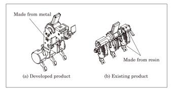
Fig.8 Opening and closing mechanism
