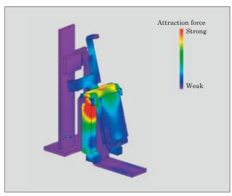
Fig.10 Examination of attraction force of electromagnetic tripping mechanism by magnetic field analysis
