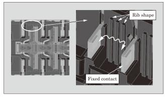
Fig.5 Frame rib shape
