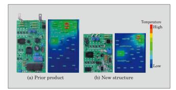
Fig.10 Thermal analysis of printed circuit board
