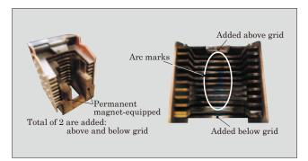
Fig.9 Status of arc-extinguishing chamber after interruption test
