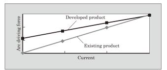
Fig.11 Effect of adding permanent magnet
