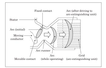
Fig.14 Schematic diagram of breaking structure in developed product
