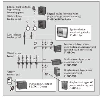
Fig.2 Application configuration diagram of "F-MPC Series"
