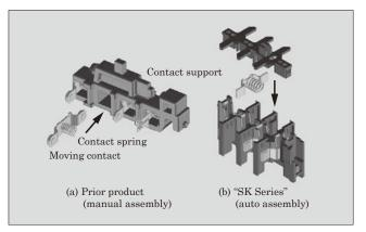
Fig.6 Contact support assembly
