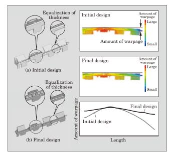
Fig.12 Resin flow analysis of crossbar
