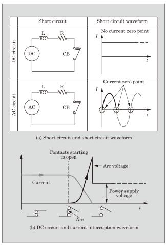
Fig.5 Current breaking and arc voltage
