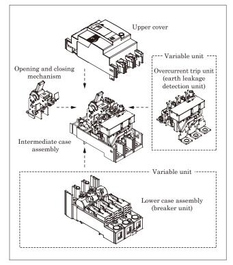
Fig.7 Modular structure of each functional unit
