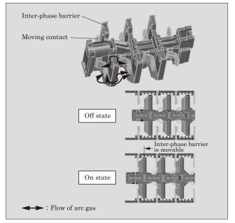
Fig.4 Barrier structure of movable parts of contact
