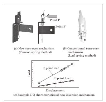
Fig.3 Turn-over mechanism
