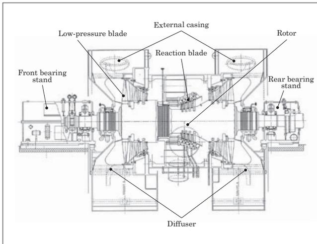
plant have changed with age. This geothermal steam turbine began operation in 1988, and as a result of changes in the steam conditions due to the long-term operation, a decrease in turbine efficiency was observed and optimization of the power generating equipment had been required.
