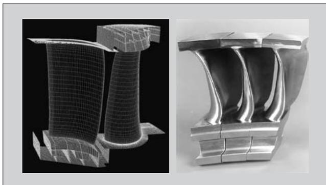
performance are used. Lean-radial stationary blades that are curved in the circumferential direction are used as the last stage stationary blades and realize a large improvement in efficiency (Fig. 4).
